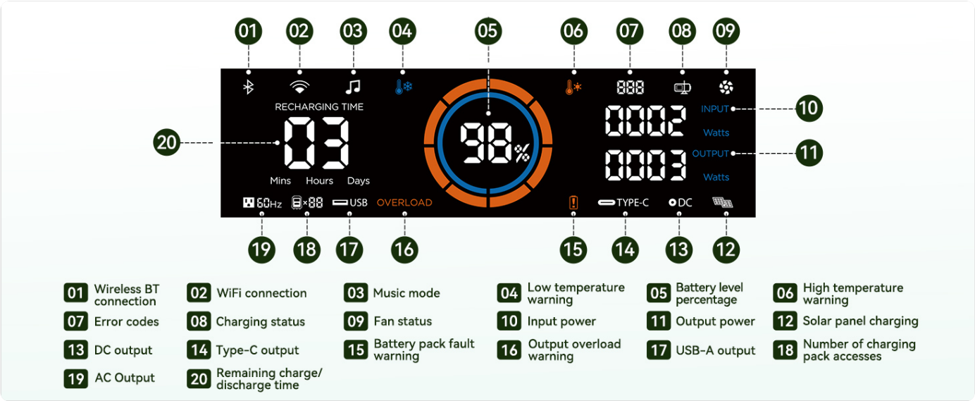
Figure 2: PowerMax 2400 Display Panel with Labeled Indicators. This diagram highlights the various icons and readings on the power
