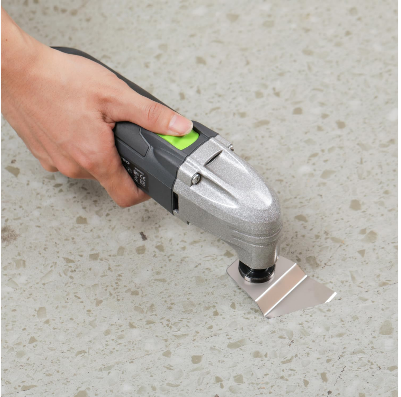
Image 5.7: The oscillating tool with a scraping blade being used on a floor surface.
