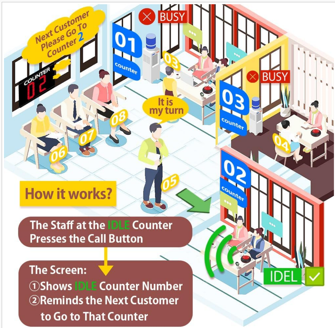
Figure 4.1: How the System Works. This diagram visually explains the process of calling a customer to an idle counter.
