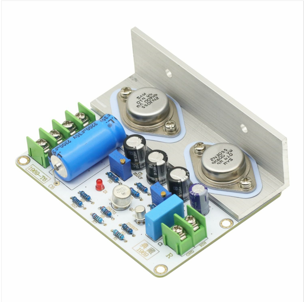
Figure 4: Close-up of the amplifier board, indicating the location of adjustable components like KT2 (W202) for current adjustment.
