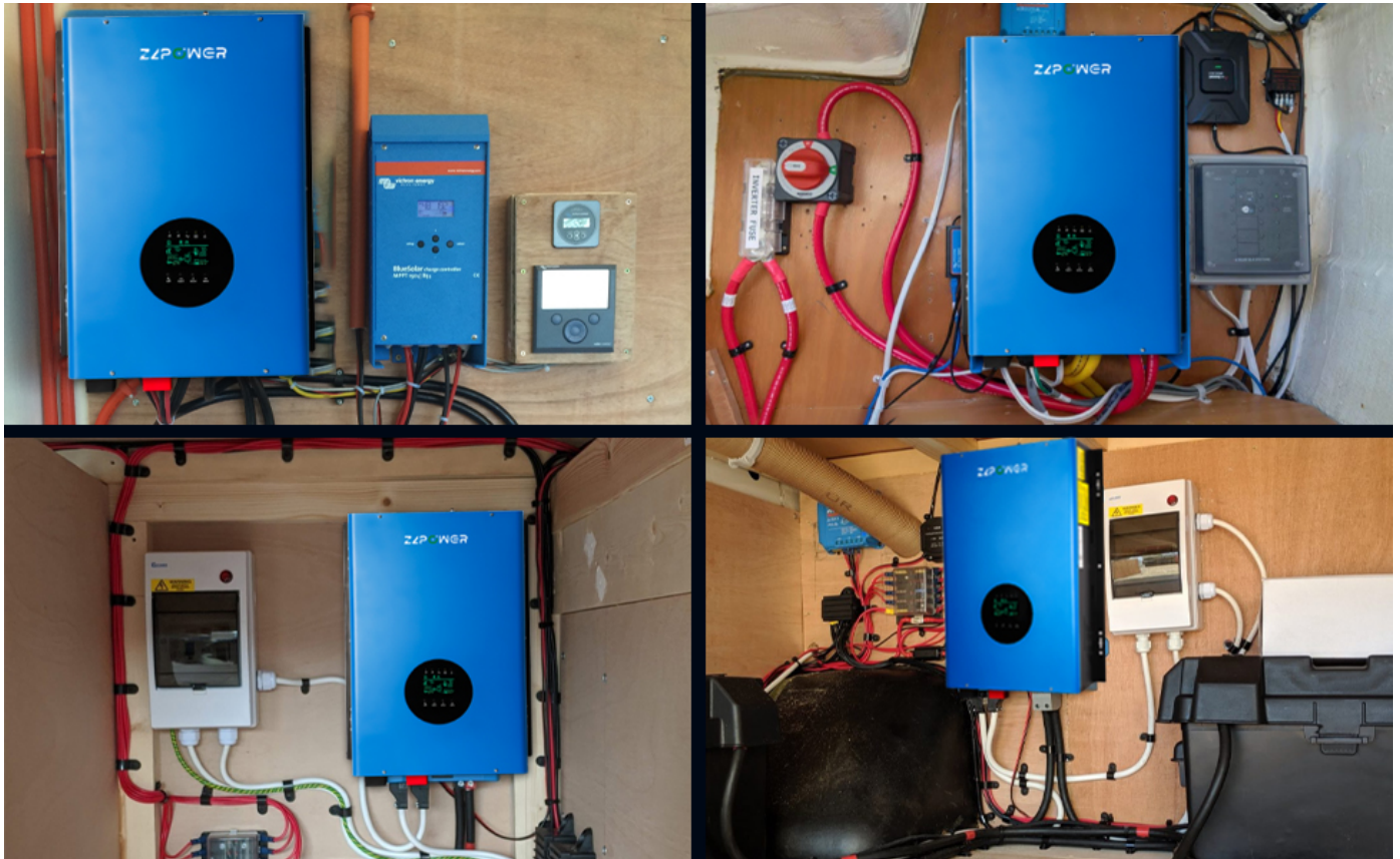
Figure 5.2: Example Installation Setups
