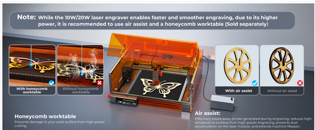
Image 5.6: Benefits of using a honeycomb worktable and air assist.
