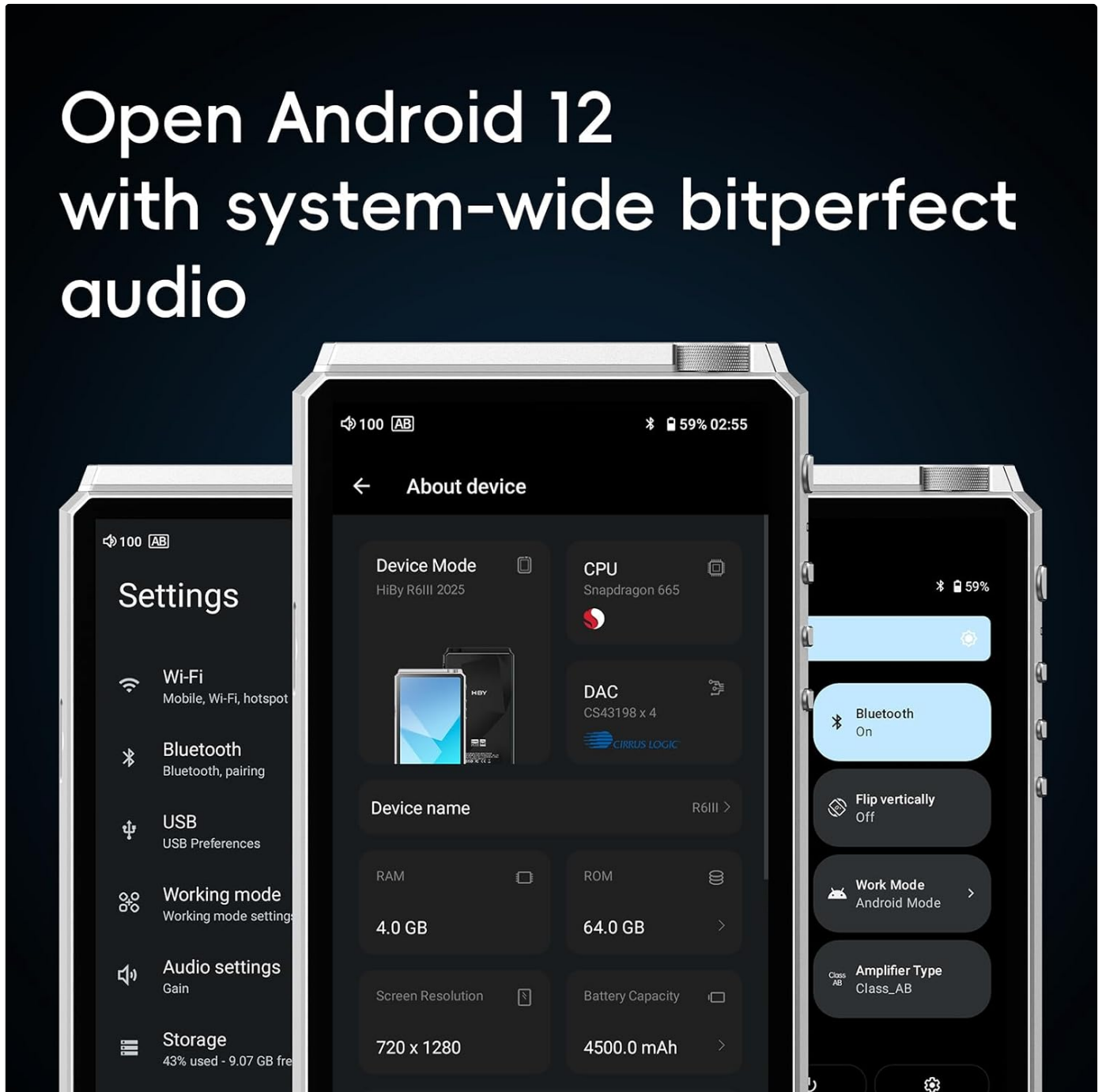
Image 4.1: The HiBy R6III 2025 running Open Android 12, showing device information and settings, including CPU (Snapdragon 665), DAC (CS43198 x 4), RAM (4.0 GB), ROM (64.0 GB), Battery Capacity (4500.0 mAh), and Amplifier Type (Class_AB).
