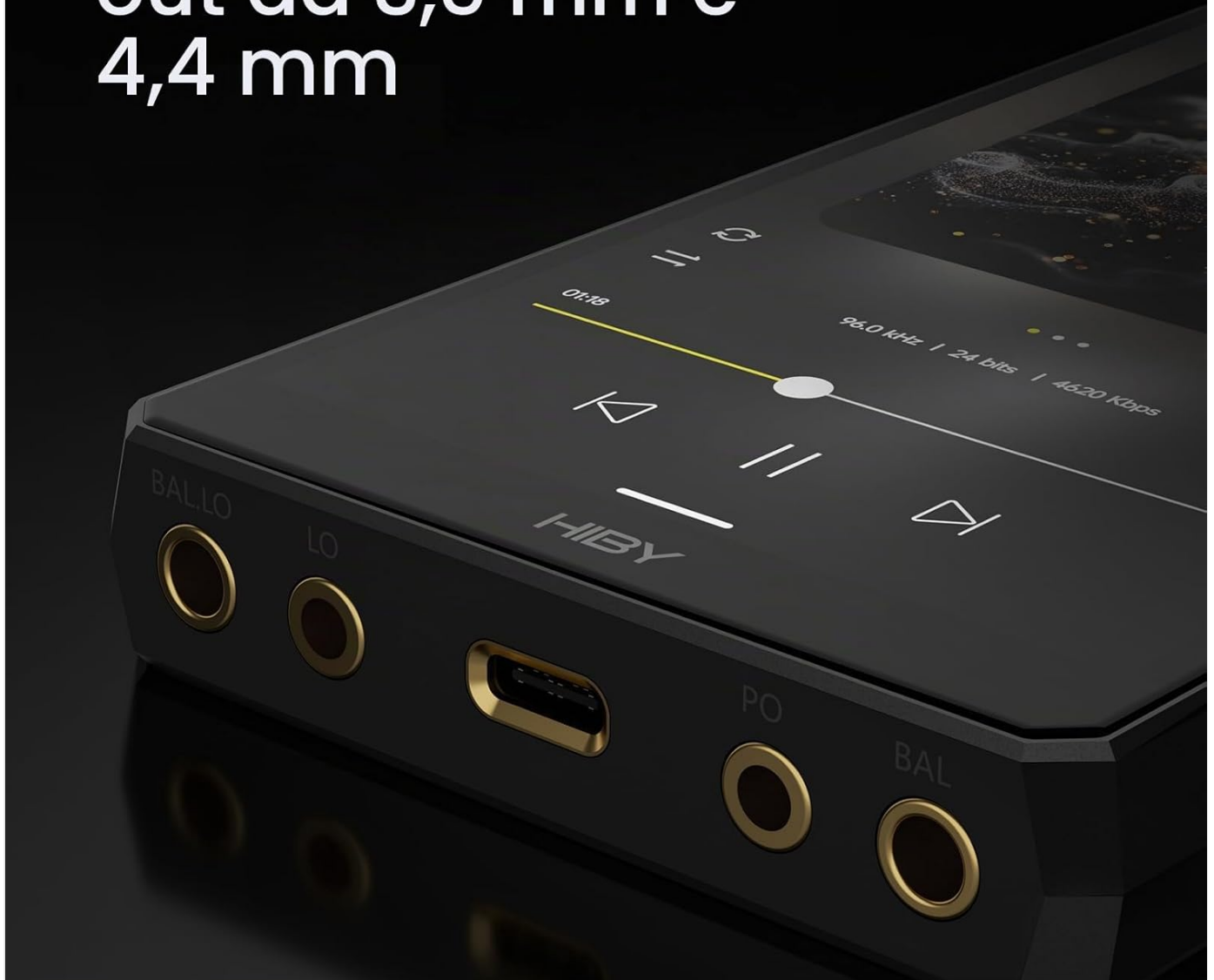
Image 3.2: Close-up view of the HiBy R6III 2025's audio output ports, showing the 3.5mm and 4.4mm headphone and line out connections.
