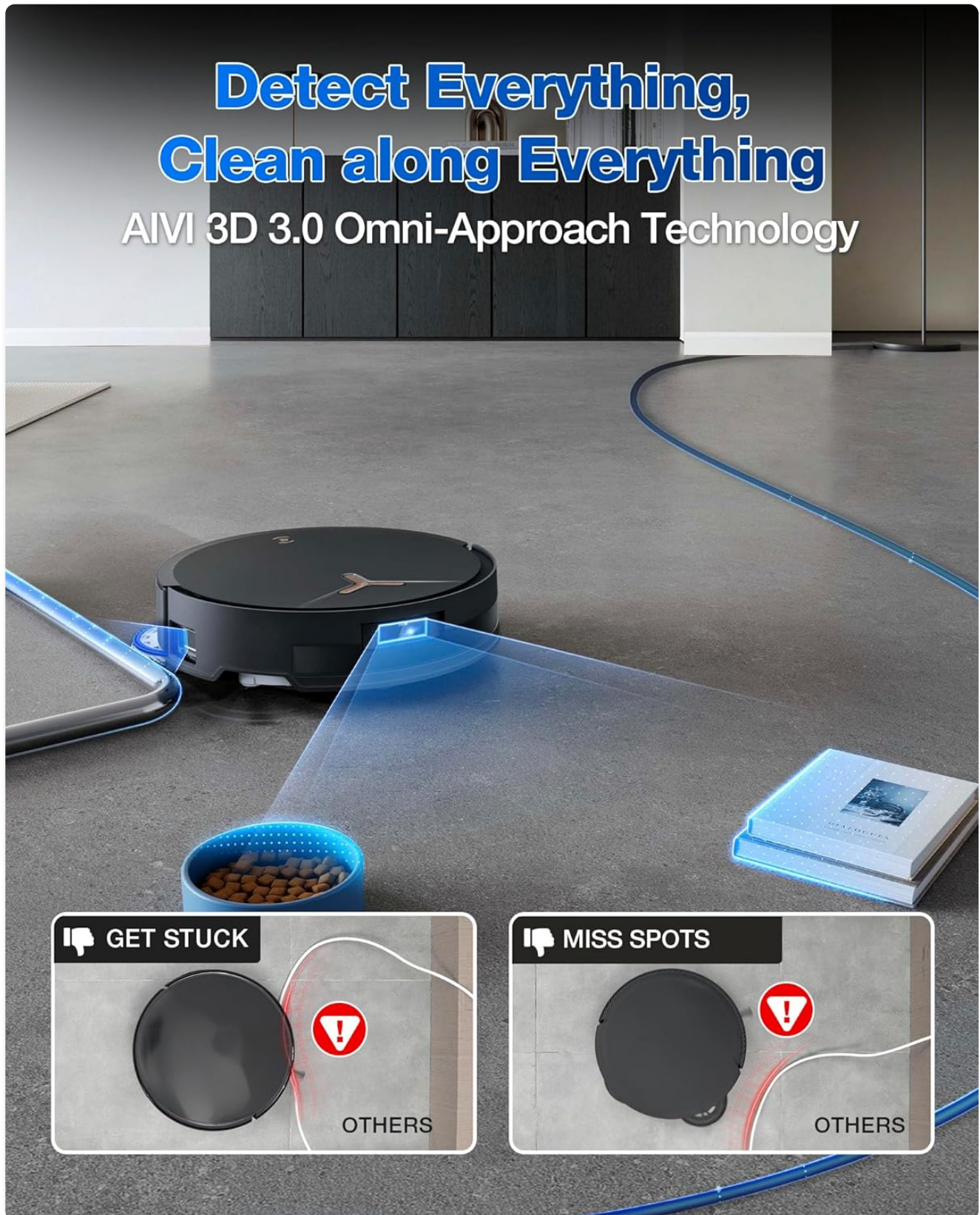
Figure 3.3: The DEEBOT T50 MAX PRO Omni demonstrating its AIVI 3D 3.0 obstacle avoidance technology, navigating around common household items.
