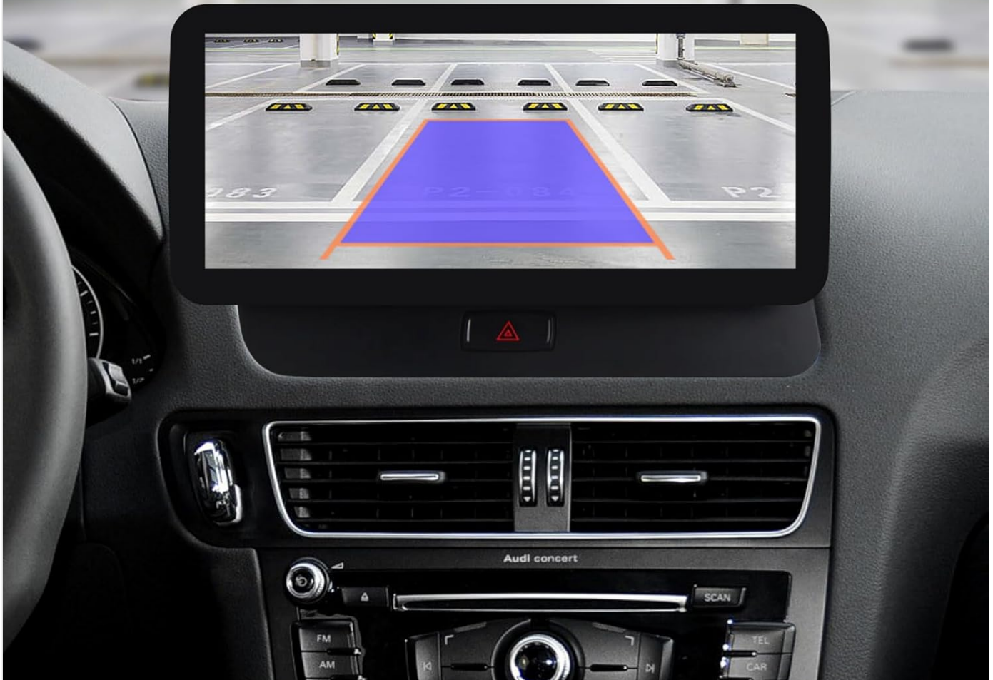
Image 5.4.1: The car radio displaying the reversing camera feed with dynamic parking guidelines, assisting the driver during parking maneuvers.
