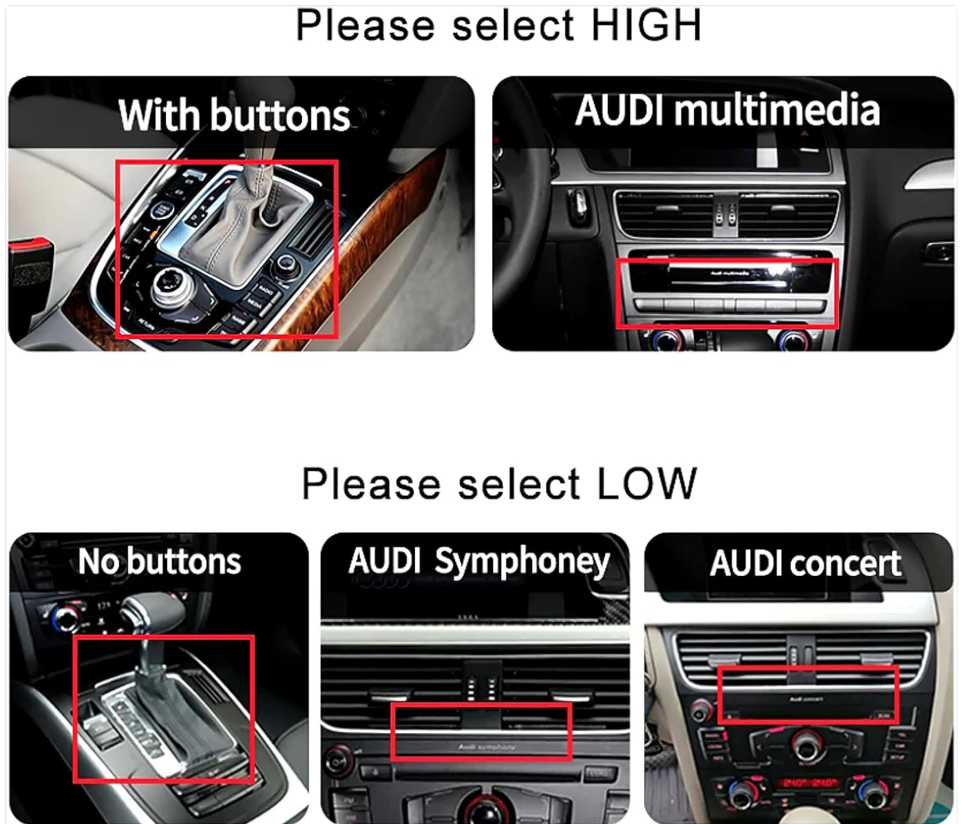
Image 3.1.1: Visual guide to distinguish between "HIGH" and "LOW" system configurations in Audi Q5 (2009-2016) vehicles. "HIGH" systems typically feature multimedia buttons, while "LOW" systems may have "AUDI Symphony" or "AUDI concert" labels without extensive multimedia controls.
