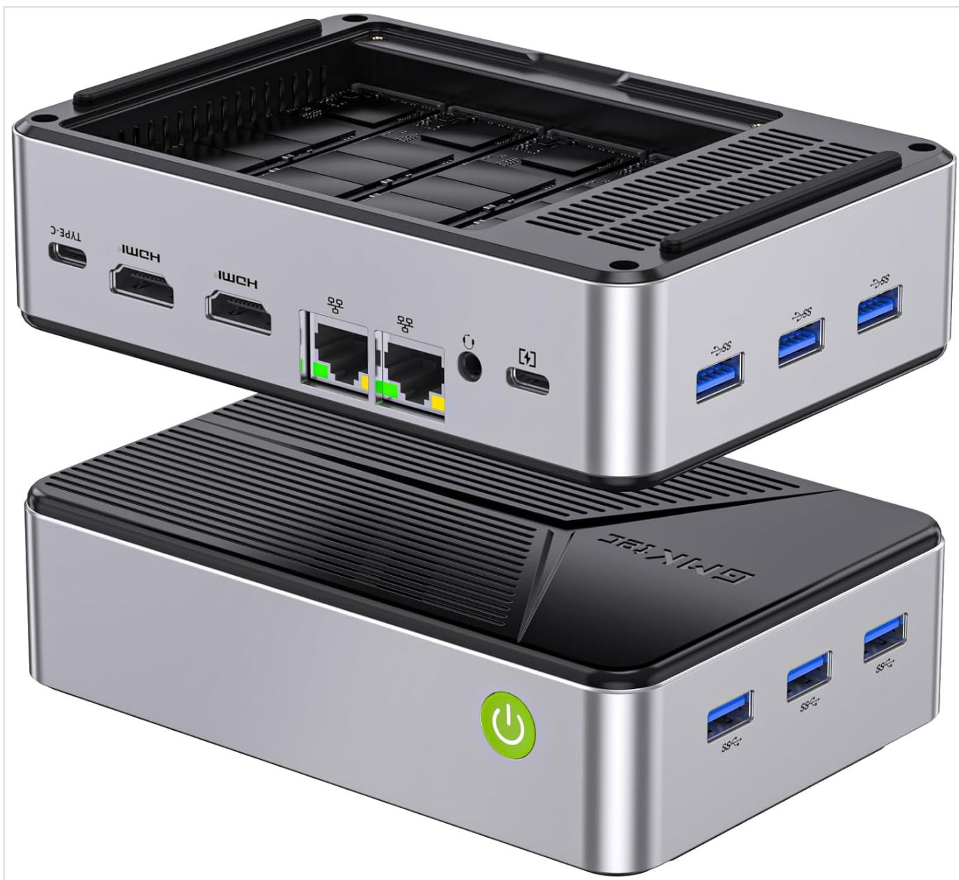
Figure 2.1: GMKtec G9 Mini PC with its top cover removed, illustrating the internal layout and accessible ports including USB-C, HDMI, Ethernet, and USB 3.2 ports.
