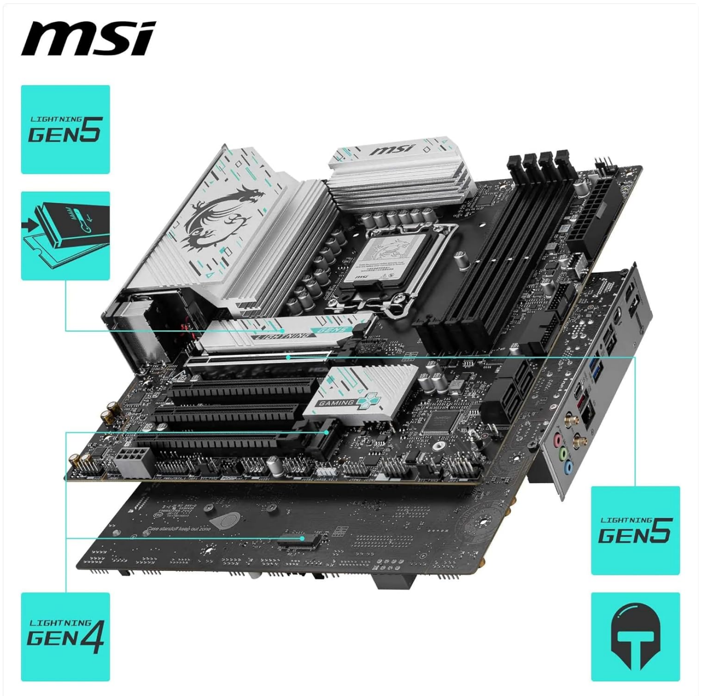
Figure 2.3: An exploded diagram illustrating the placement of PCIe 5.0 x16 and M.2 Gen5/Gen4 slots on the motherboard.
