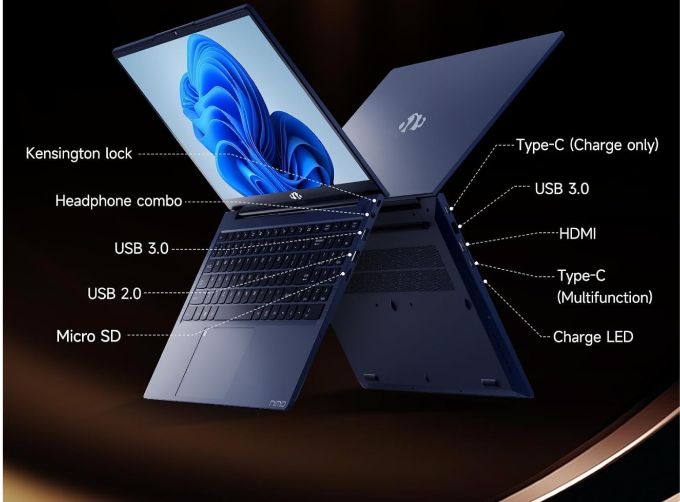
Figure 8: Diagram illustrating the various ports available on the NIMO laptop, including Kensington lock, Headphone combo, USB 3.0, USB 2.0, Micro SD, HDMI, and Type-C (Multifunction/Charge only).
