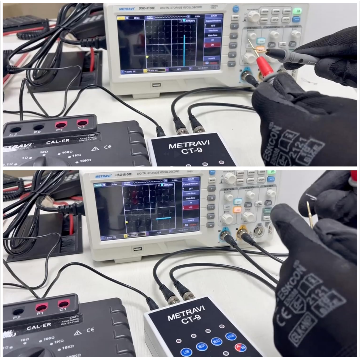
Figure 4.1: The Metravi CT-9 connected to a digital oscilloscope via BNC cables, ready for component testing.
