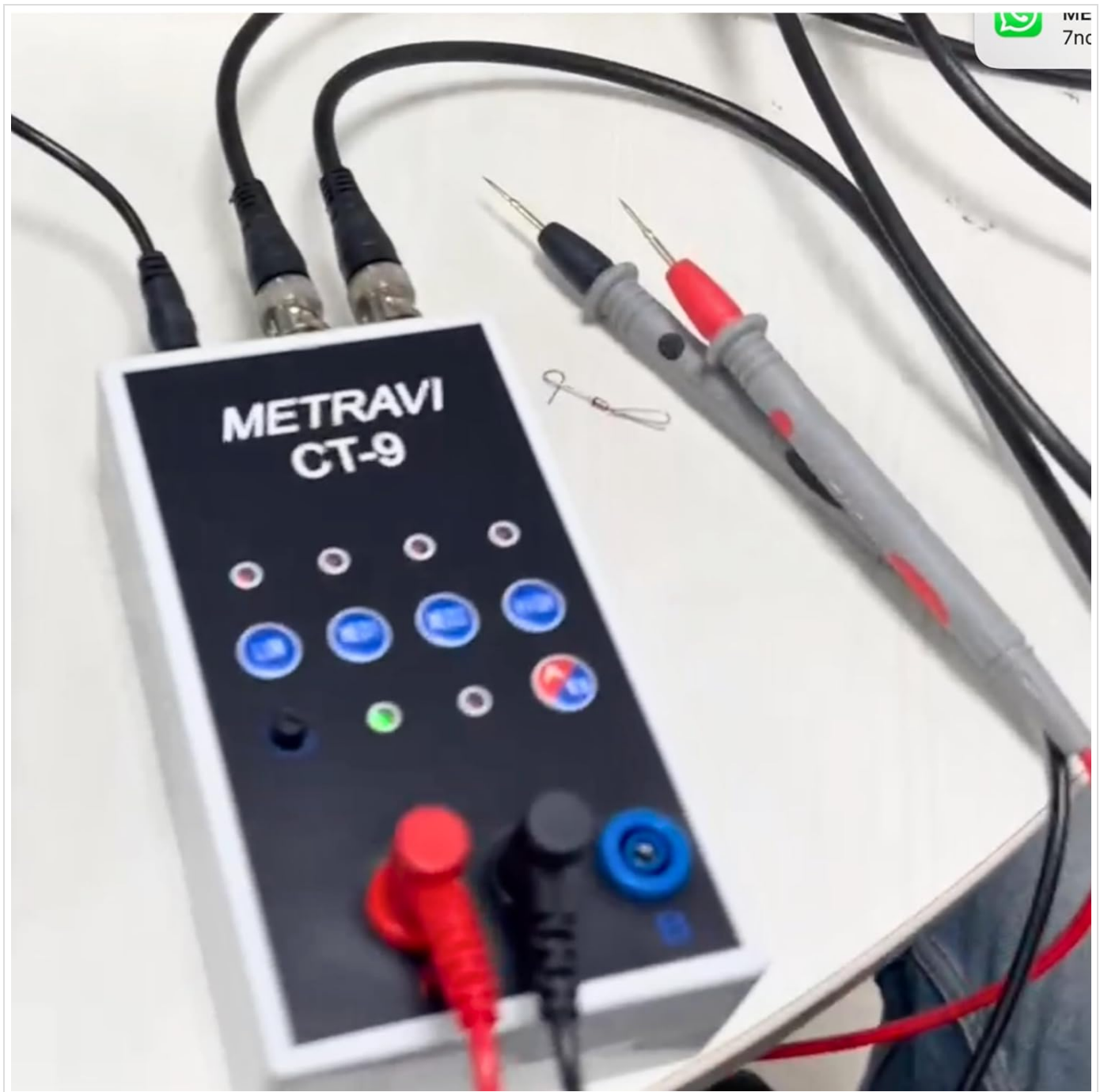
Figure 4.2: Close-up view of the Metravi CT-9 with test leads connected and BNC cables running to an oscilloscope, demonstrating a typical setup.
