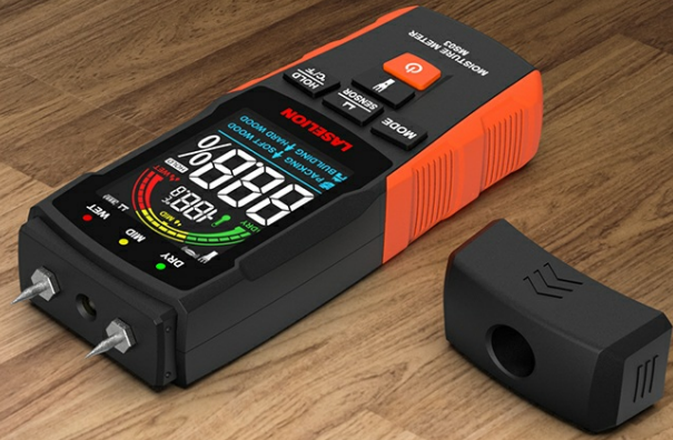
Image: The LASELION MS03 moisture meter displaying its four testing modes: Soft Wood, Hard Wood, Building Mode, and Packing Mode, with examples of materials for each category.
