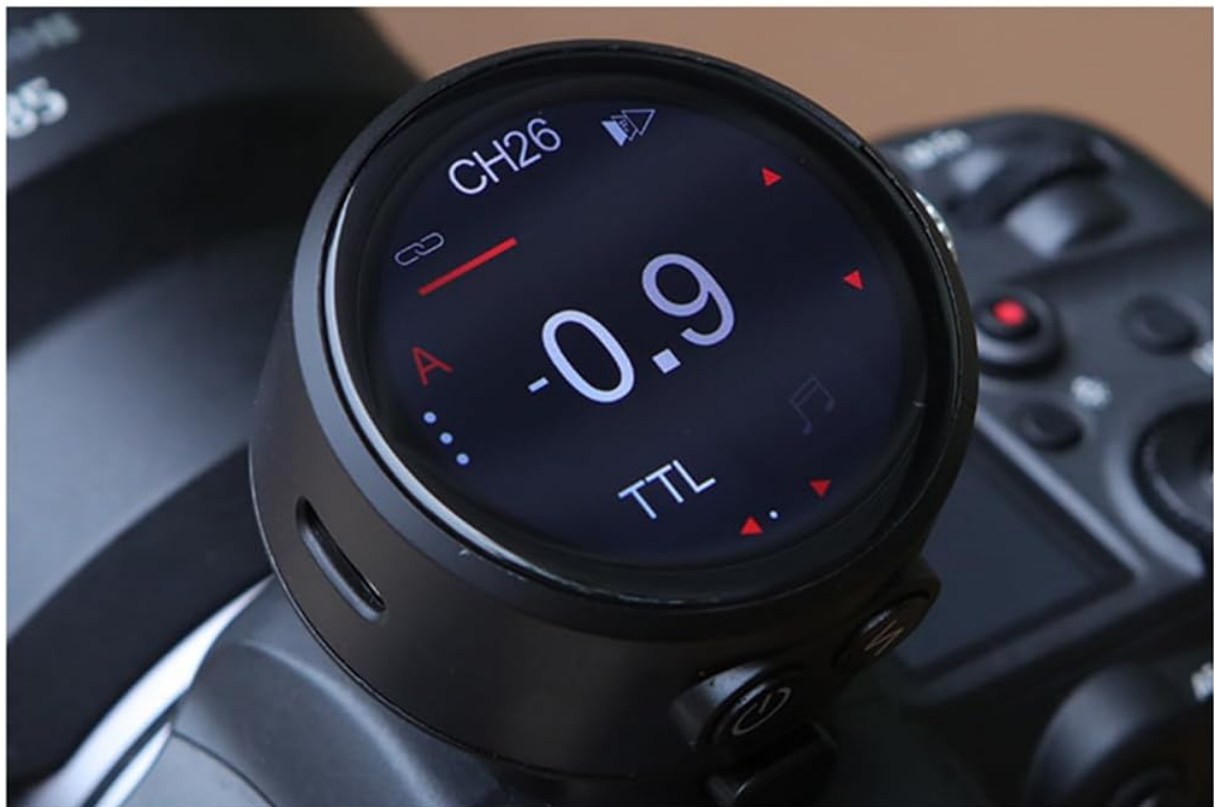
Image 6.1: The TR-Q8 display indicating TTL mode and exposure compensation settings.
