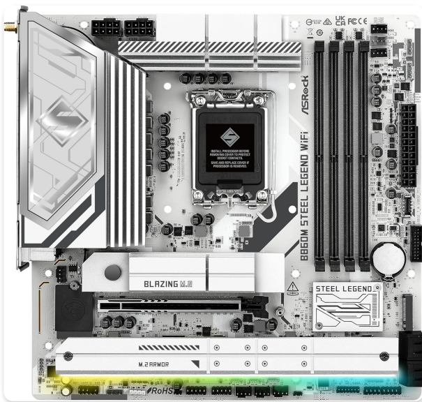
Image: Front view of the ASRock B860M Steel Legend WiFi 6E Motherboard, showcasing the CPU socket, RAM slots, and heatsinks.
