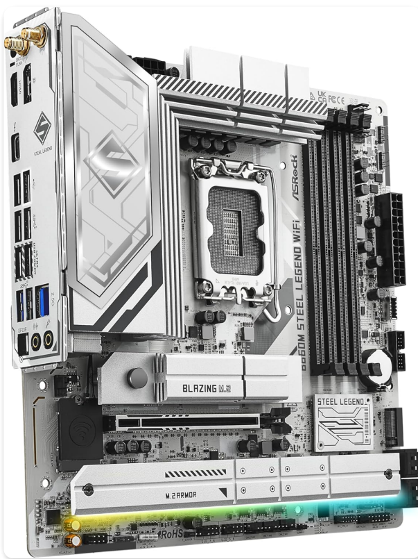
Image: Angled view of the ASRock B860M Steel Legend WiFi 6E Motherboard, highlighting the M.2 slots with heatsinks.
