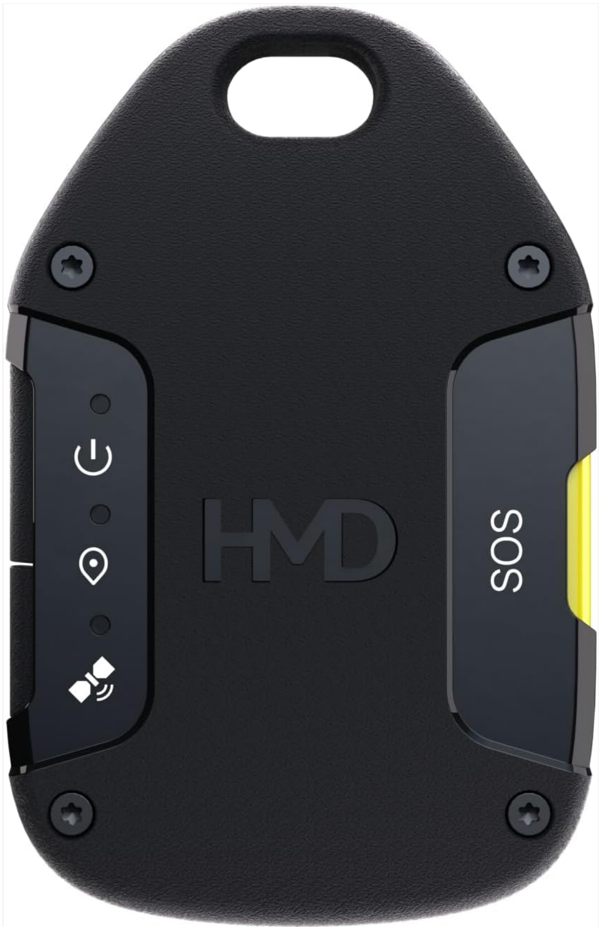
Figure 1: Front view of the HMD OffGrid Satellite Communicator, showing the HMD logo and indicator lights.
