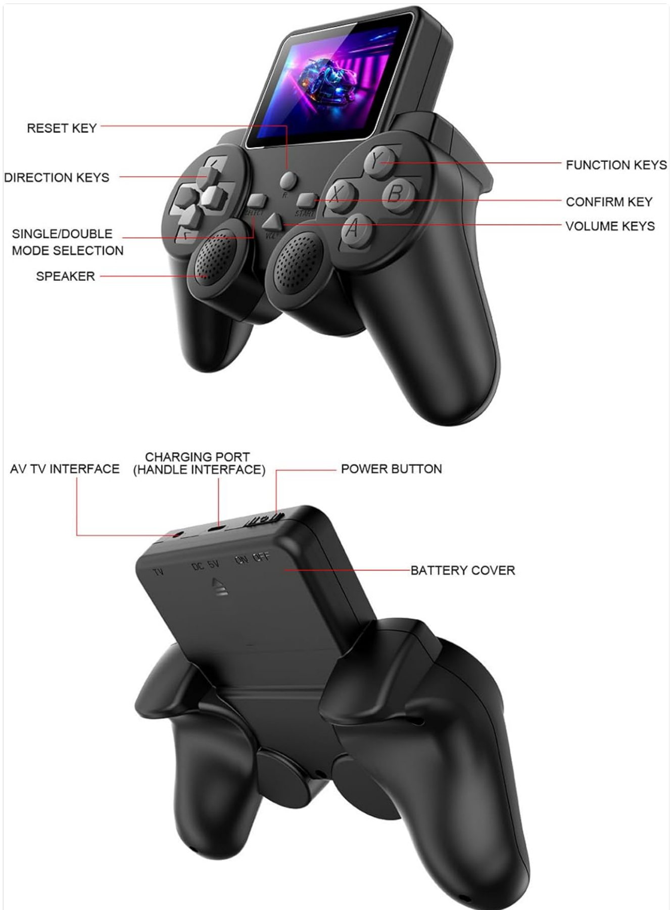
Image 3.1: Labeled diagram illustrating the buttons, ports, and features of the VBESTLIFE Handheld Game Console.
