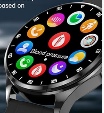
Figure 2.2: The 1.43-inch AMOLED HD screen with 466*466 resolution and various dynamic menu styles.
