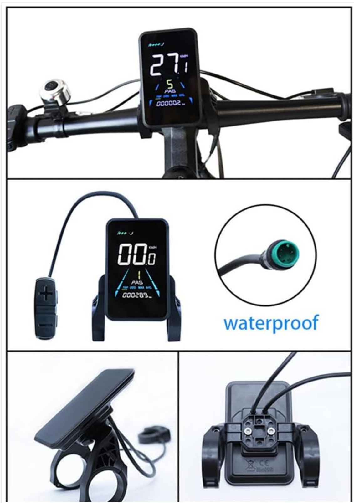
Image: A comprehensive view of the YL81F K5 display, illustrating its vibrant color screen and the integrated K5 button controls.
