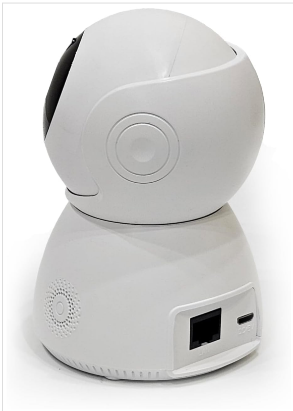
Figure 3.3: Back View. Displays the speaker grille and DC 5V power input.
