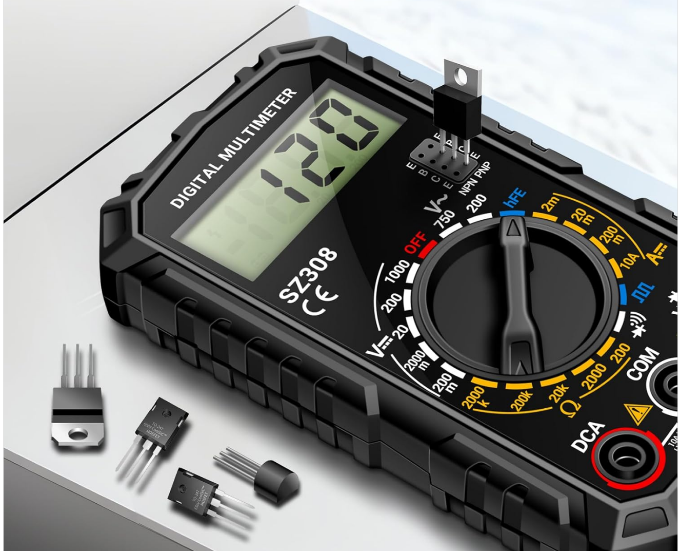
Figure 6.2: Performing an hFE (transistor gain) test.
