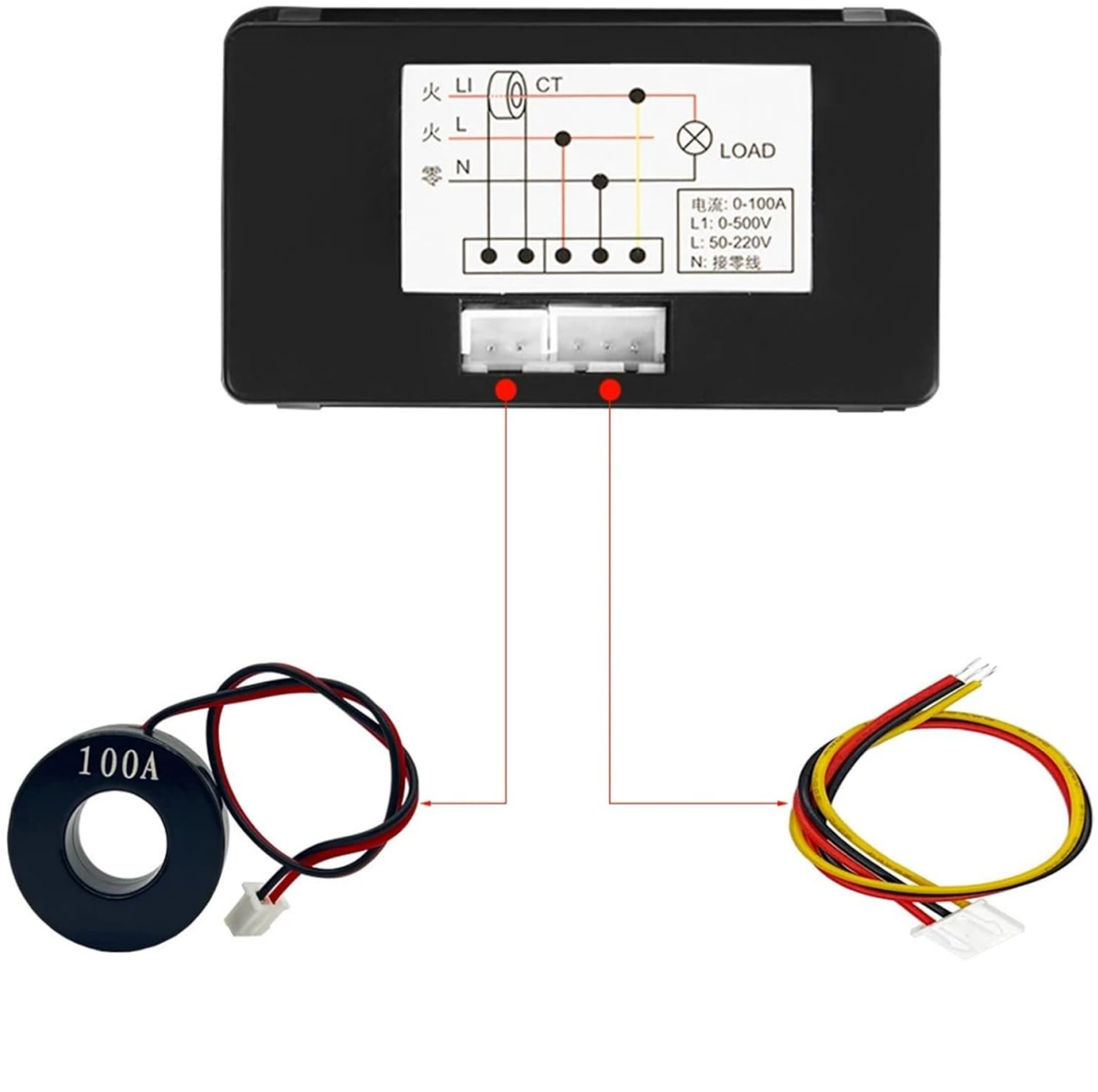
Figure 4: Wiring diagram for the KWS-AC305 meter. Connect the main power supply (L, N) to the meter's input terminals. The current transformer (CT) should be installed around the load wire (L) to measure current. The load is connected to the output terminals.
