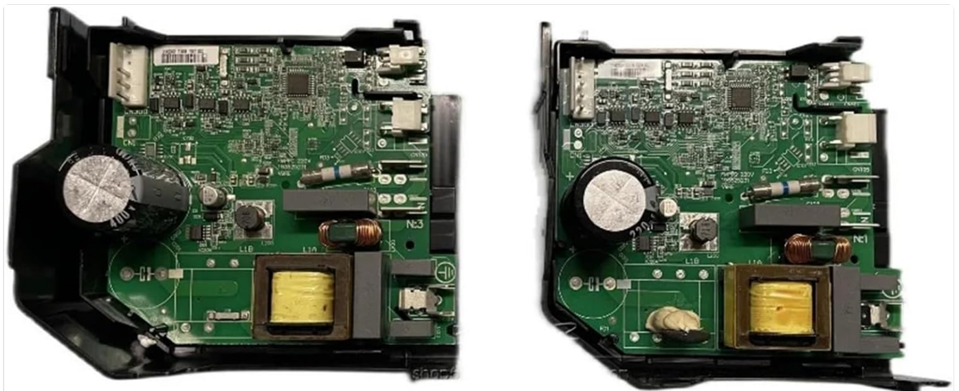
Figure 4: Comparison of two control boards, illustrating that the internal structure is consistent across compatible models, which is important for universal
