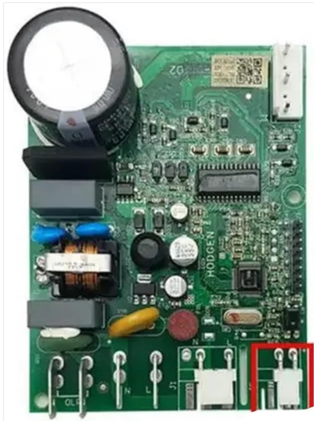
Figure 1: Top view of the BTJCRLEB Refrigerator Inverter Board (VTB1113Y, JXPR-03, D2A).
