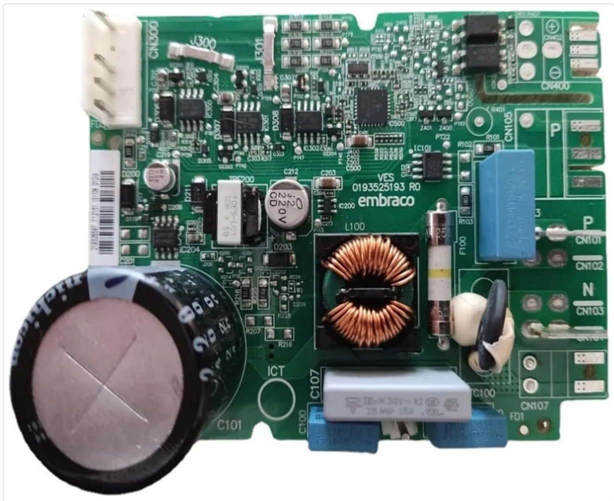
Figure 2.1: Top view of the Embraco VESD9C Refrigerator Compressor Inverter Board. This image displays the various electronic components and connectors on the circuit board.
