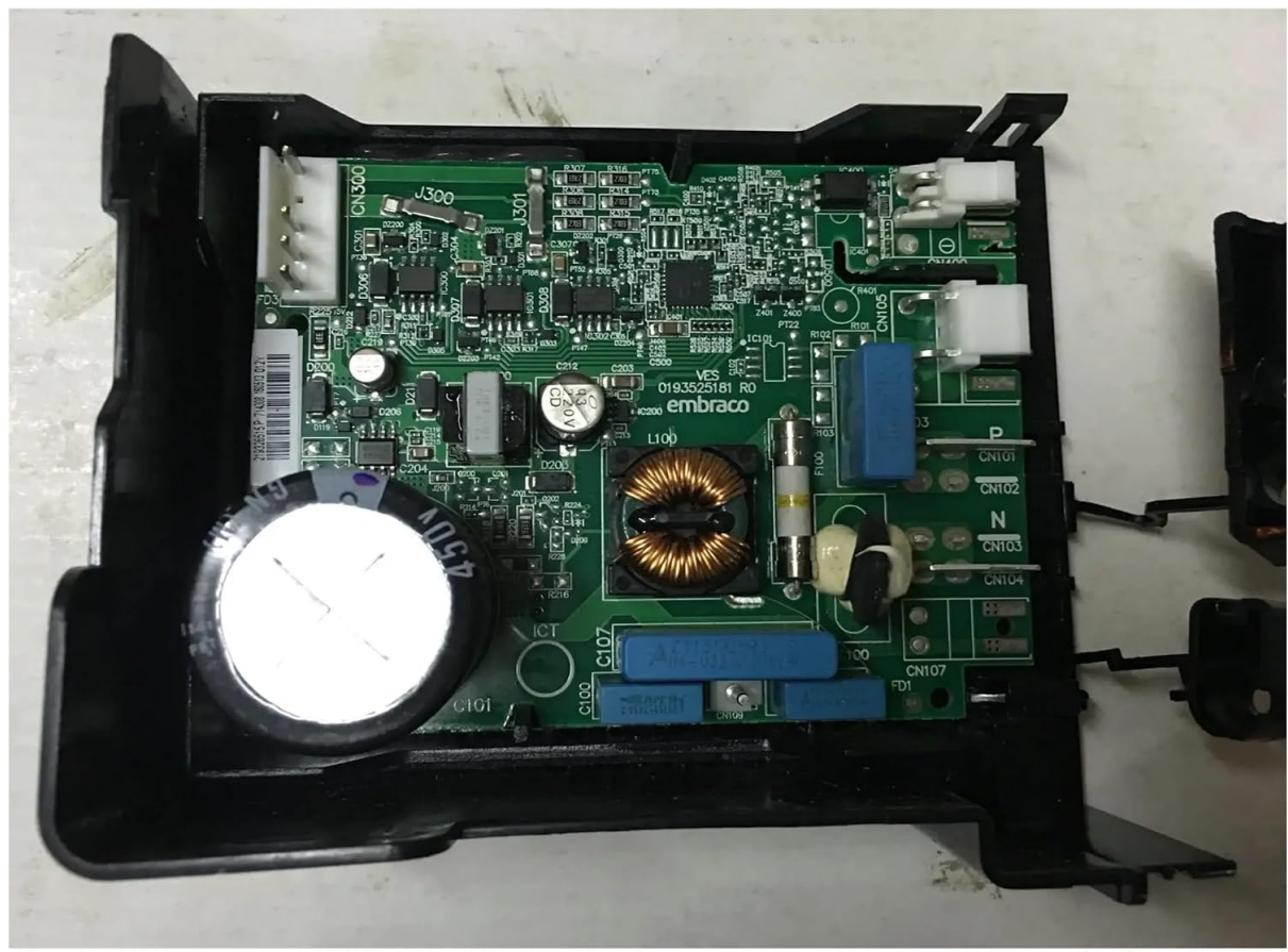
Figure 4.1: The Embraco VESD9C inverter board shown partially installed within its protective casing, illustrating the connection points.
