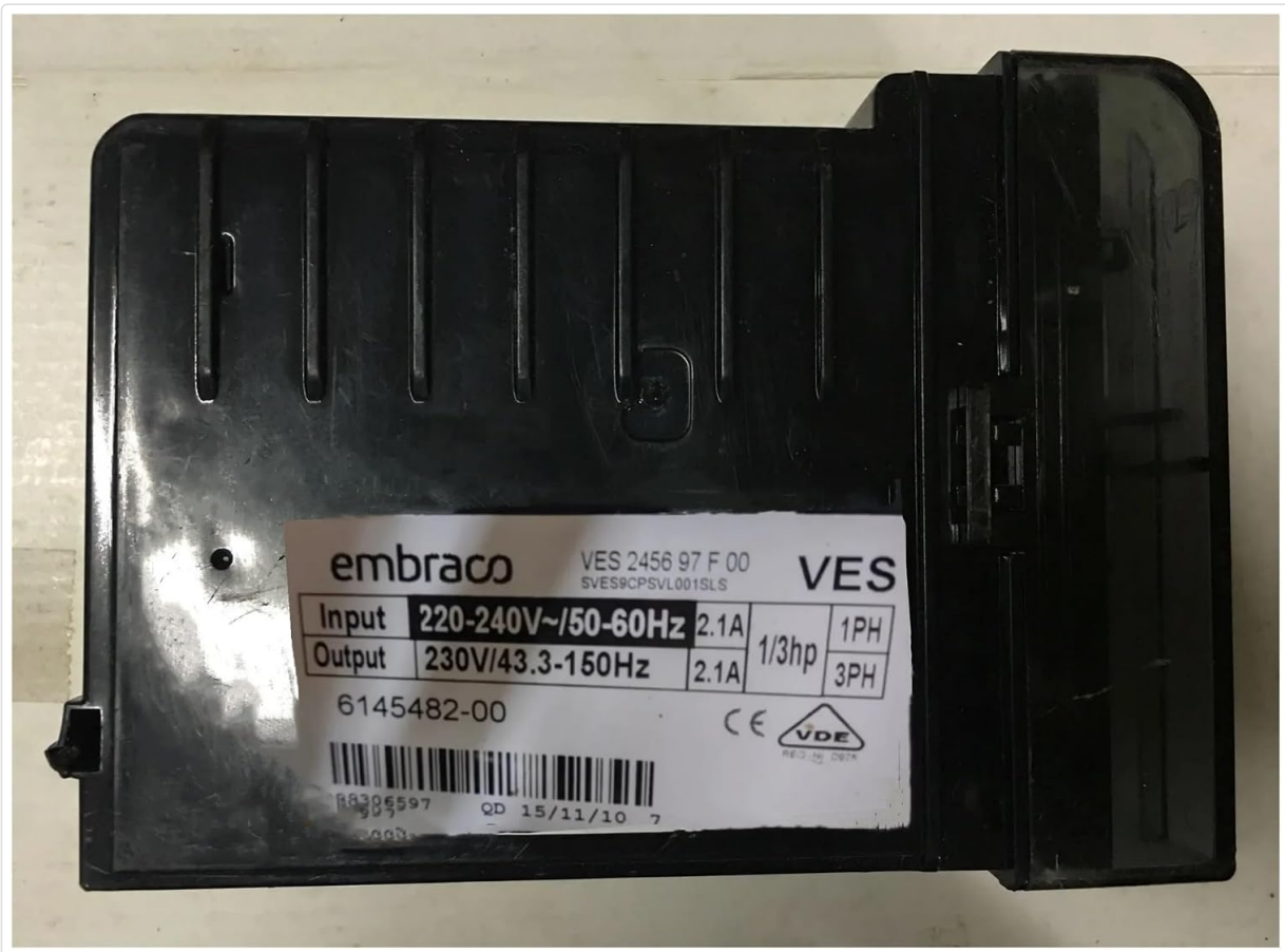
Figure 3.1: Label on an Embraco inverter board casing, showing input/output specifications and a caution regarding electric shock. Note the warning: "CAUTION: Risk of electric shock. Before touching terminals unplug system and wait 30 seconds."
