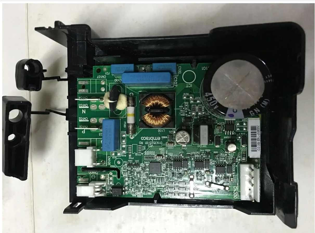
Figure 4.2: Another view of the Embraco VESD9C inverter board within its casing, highlighting different angles of the circuit board and its components.
