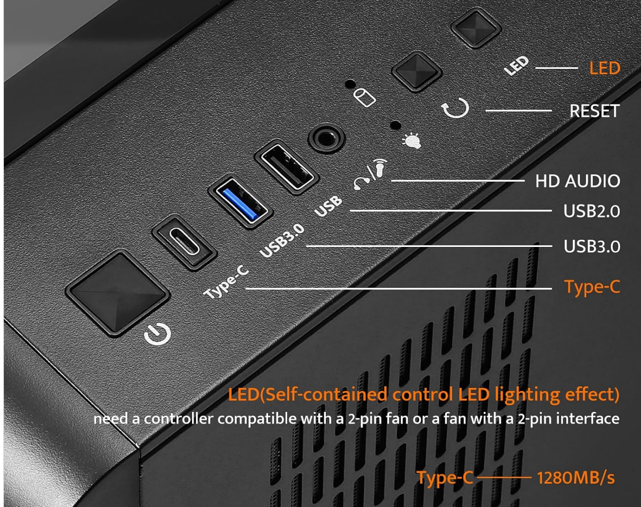
Image 5.2: The front I/O panel detailing the power, reset, and LED buttons, along with USB Type-C, USB 3.0, USB 2.0, and HD audio ports.
