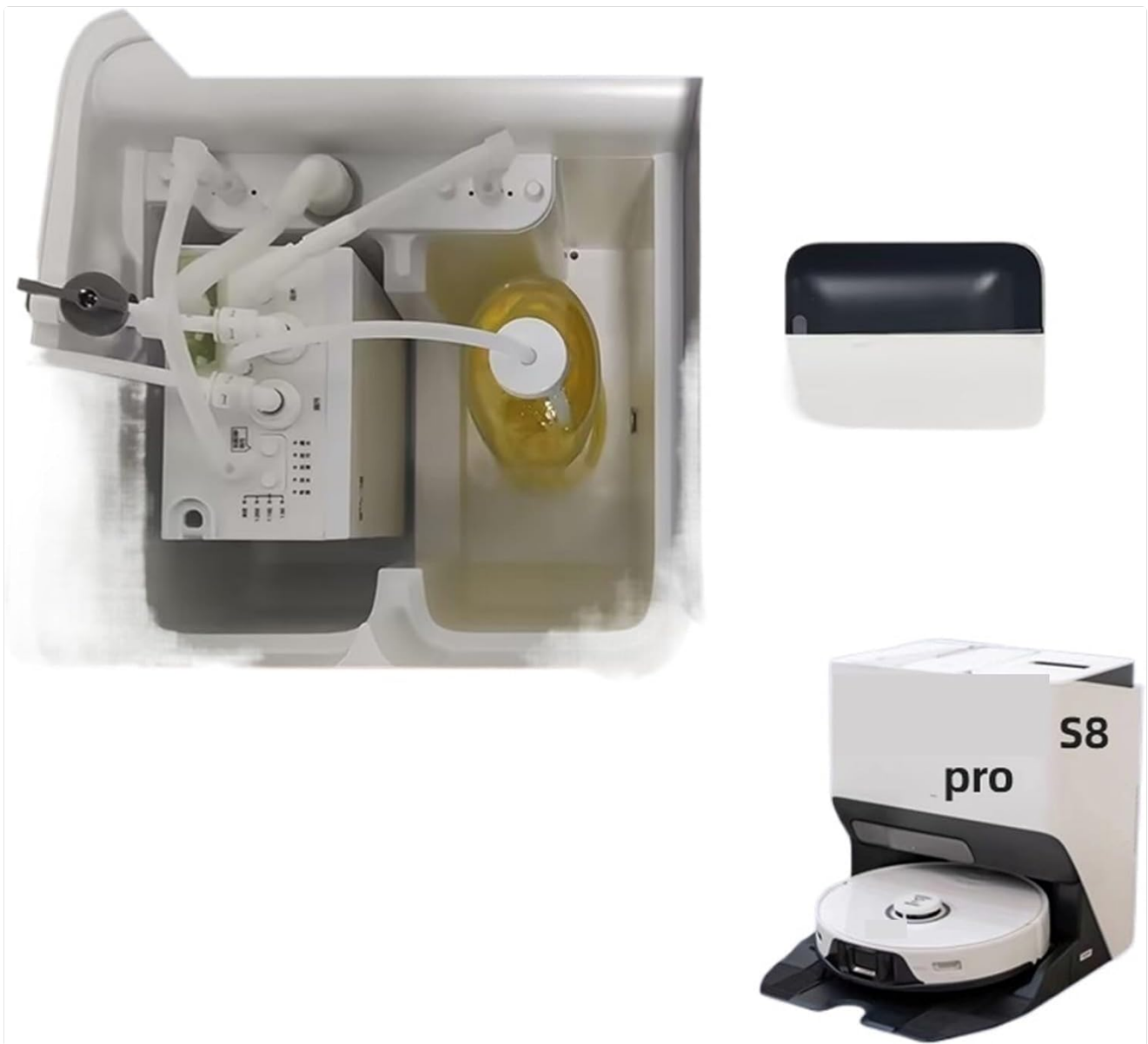
Figure 3: Detailed internal view of the water change module, highlighting the various connection points for water supply, drainage, and cleanser.
