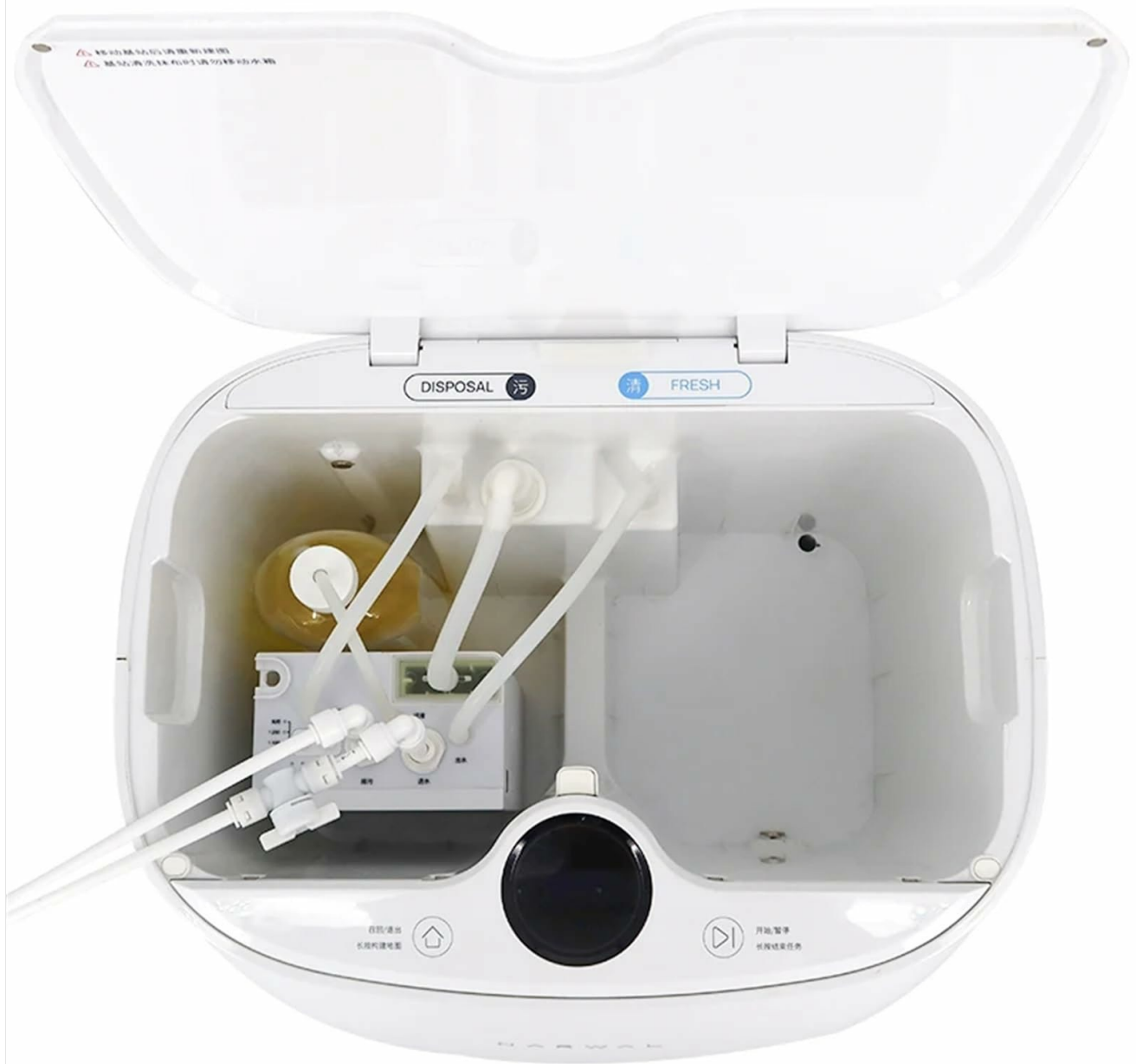
Figure 2: An overview of the robot vacuum base station with the water change kit module integrated. The module replaces the standard water tanks.
