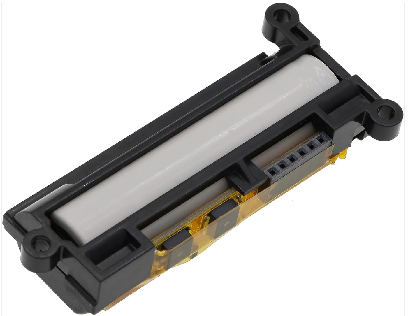
Figure 4: Side view of the battery, revealing the internal cylindrical cell and part of the circuit board.
