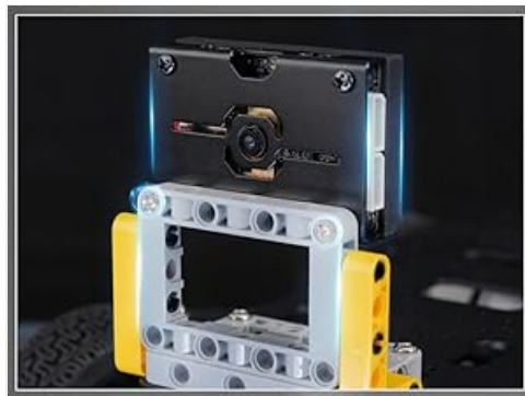
Figure 2: Powerful Hardware Features. This image highlights the robust design of the WonderMV module, showcasing its metal shell, 200W HD camera, dual communication ports, and LEGO-compatible mounting holes.
