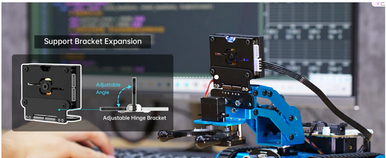
Figure 12: Support Bracket Expansion. This image illustrates the use of an adjustable hinge bracket to mount the WonderMV module, allowing for flexible positioning in projects like robotic arms.
