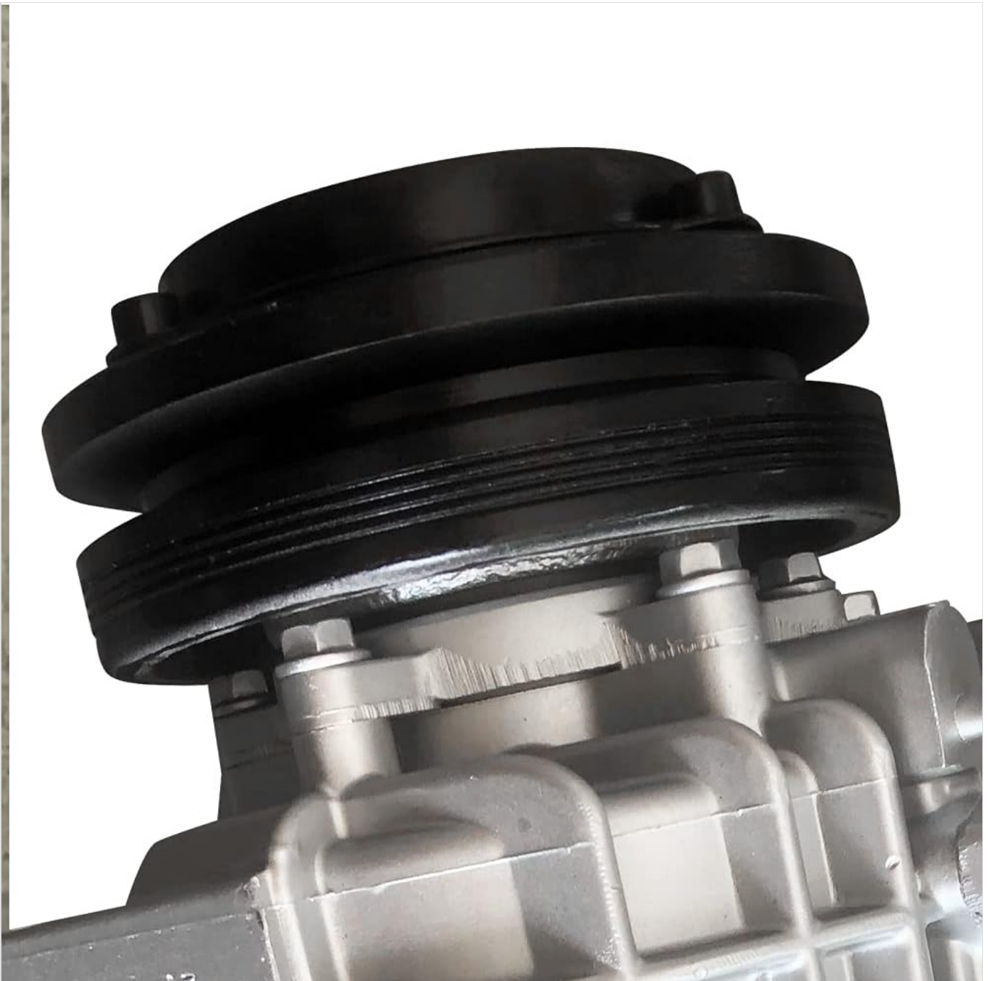
Image 3: Close-up view of the supercharger's V-pulley system. This component connects to the engine's accessory drive belt.
