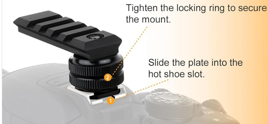
Image 4.2: Installation steps for the reflex sight onto the Picatinny base.
