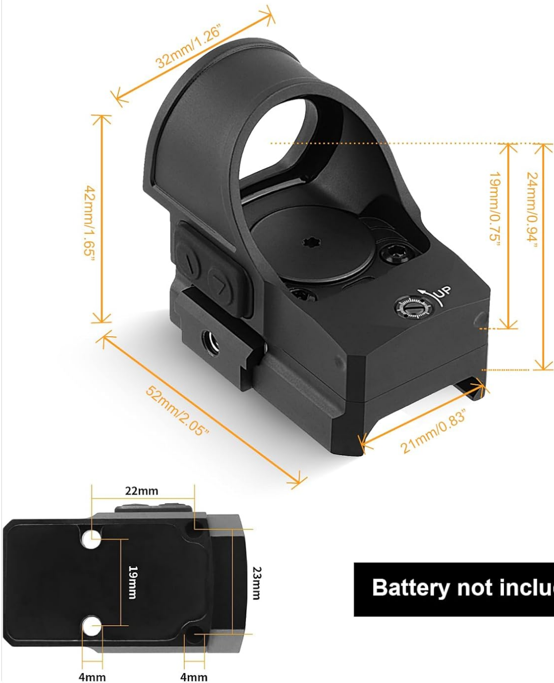
Image 8.1: Key dimensions of the FOCUHUNTER Reflex Sight.
