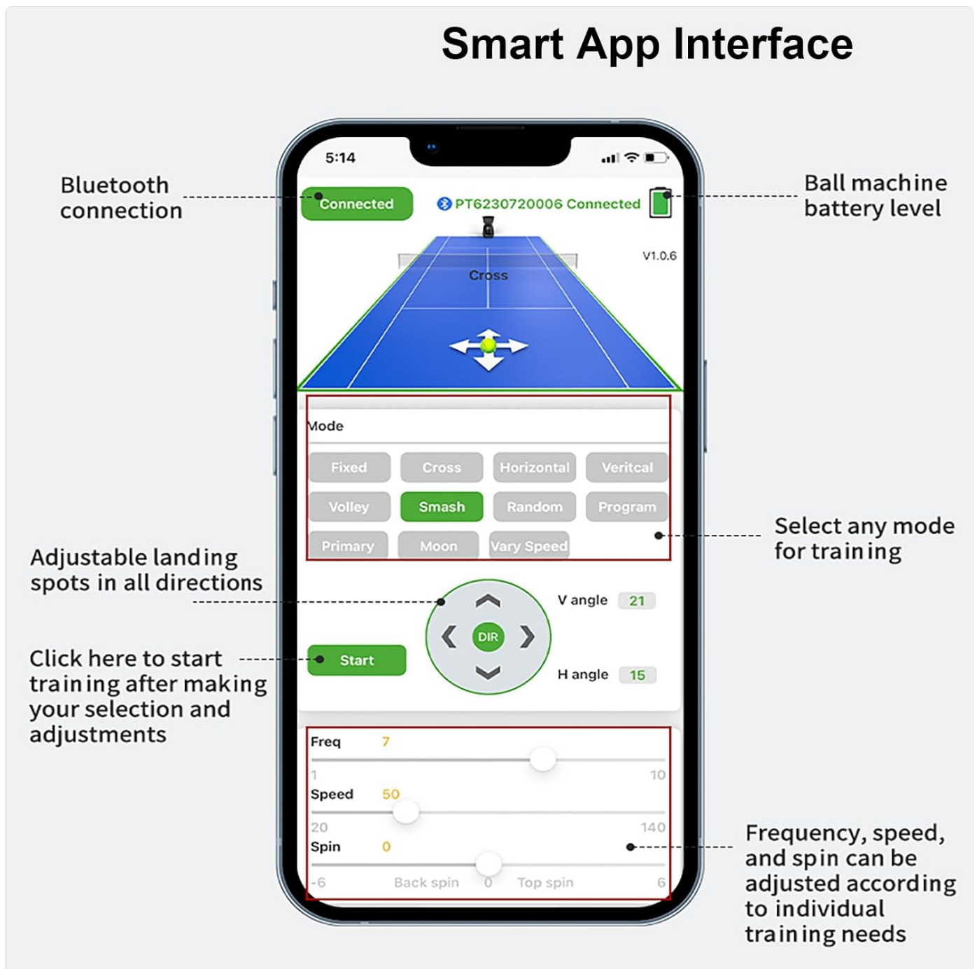
Image: A detailed view of the Smart App Interface, showing options for Bluetooth connection, battery level, adjustable landing spots, various training modes, and controls for frequency, speed, and spin.
