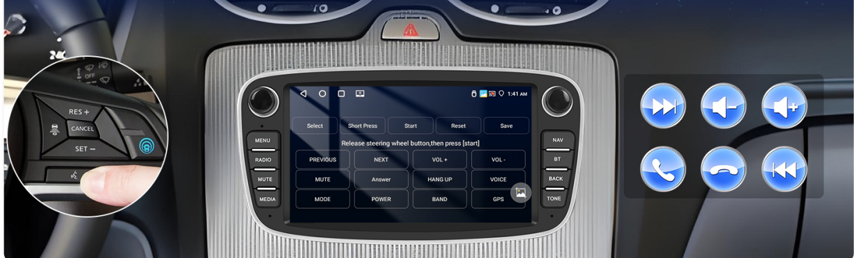
Image 3.12: The steering wheel control learning screen, indicating the path to access the learning function within the settings.
