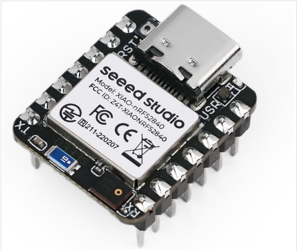
Figure 1: Top view of the Seeed Studio XIAO nRF52840 Sense (Pre-Soldered) board, showing the USB-C port and main chip.
