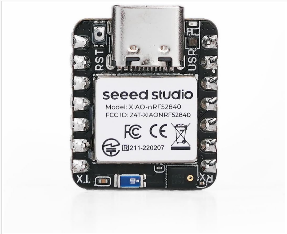
Figure 3: Close-up top view of the XIAO nRF52840 Sense, indicating the location of the reset button.
