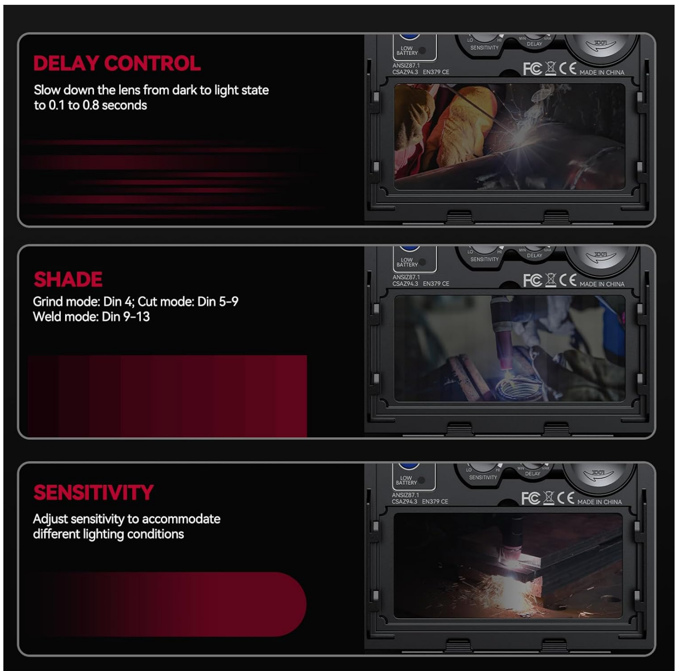
Image 4: Controls for Delay, Shade, and Sensitivity on the auto-darkening filter.
