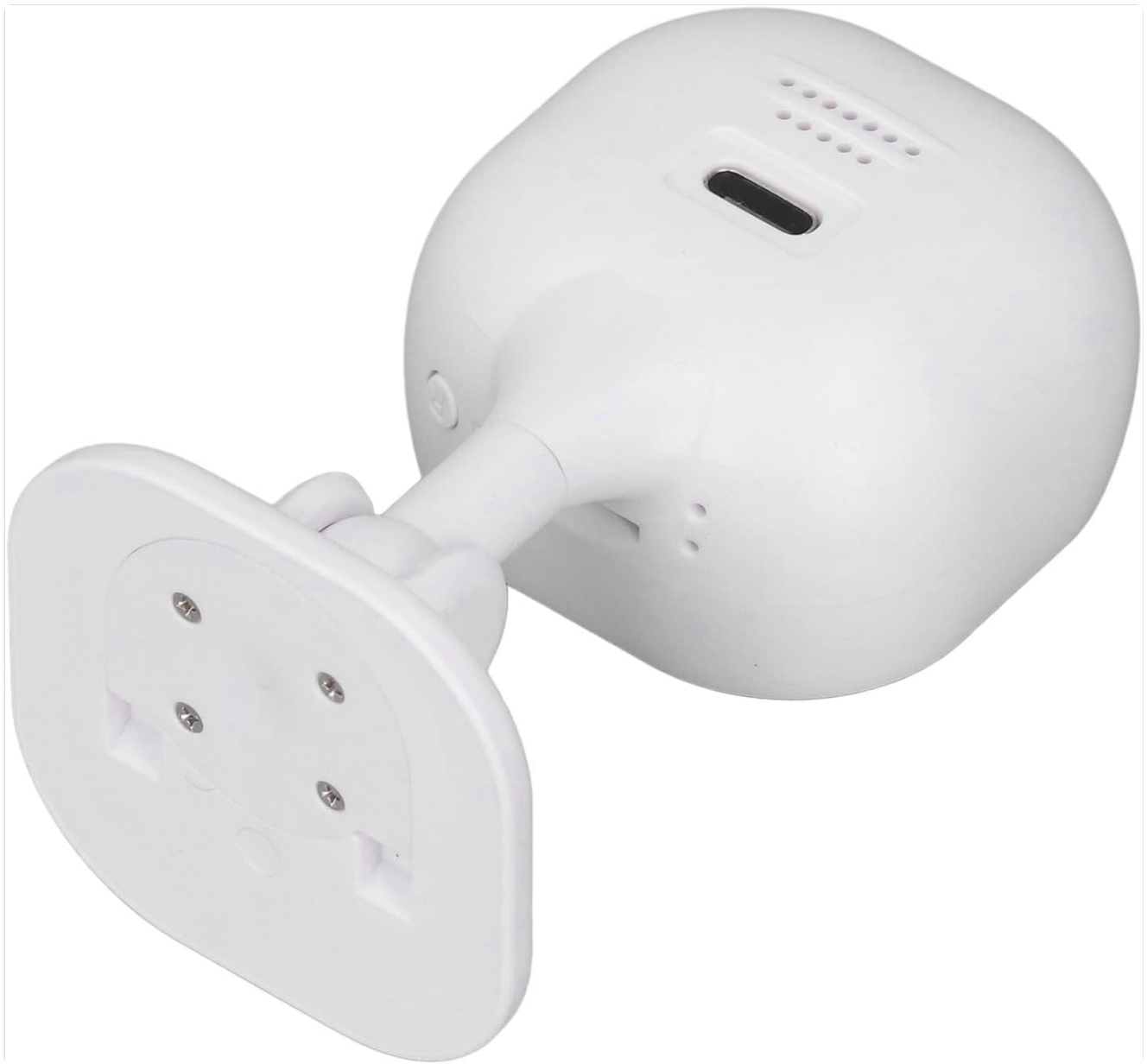
Figure 5.1: Back view of the camera, highlighting the Micro USB power input.
