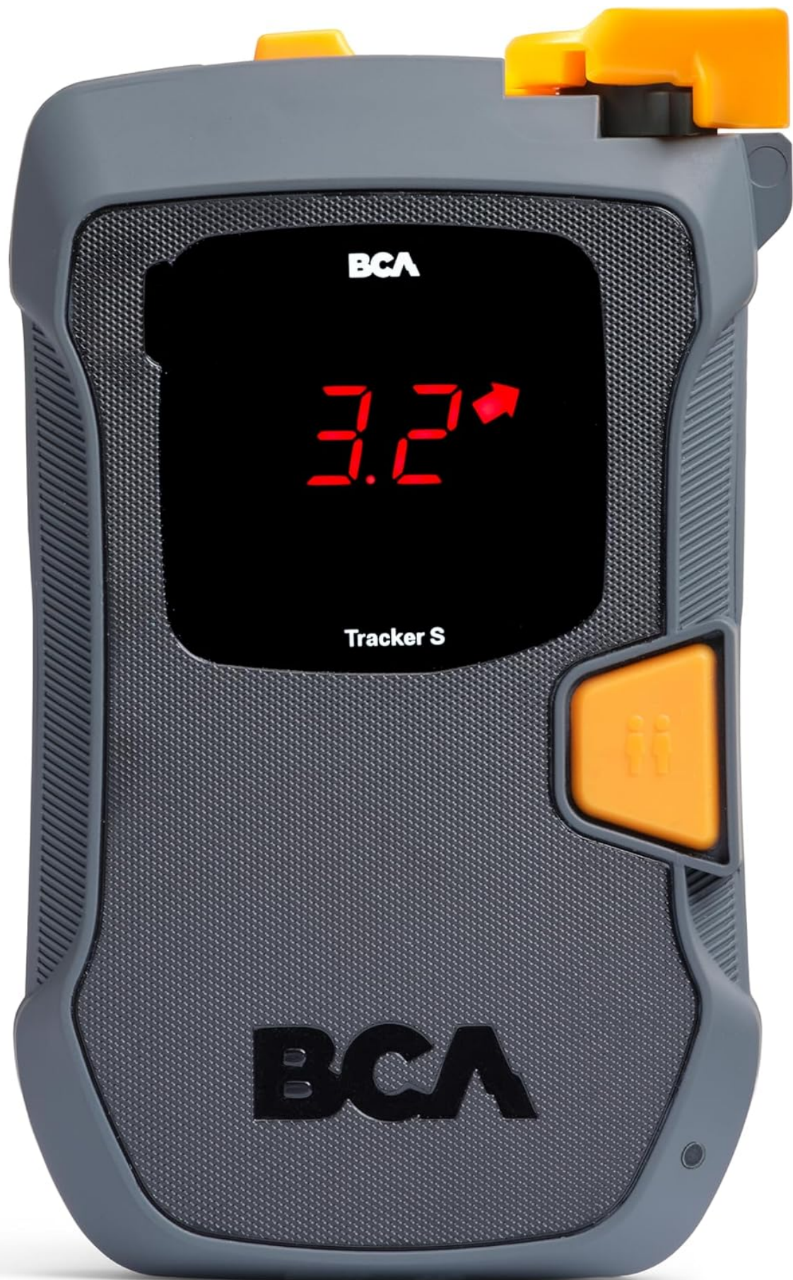
Image 3.2: Close-up of the BCA Tracker S Avalanche Transceiver display, showing distance and direction indicators.
