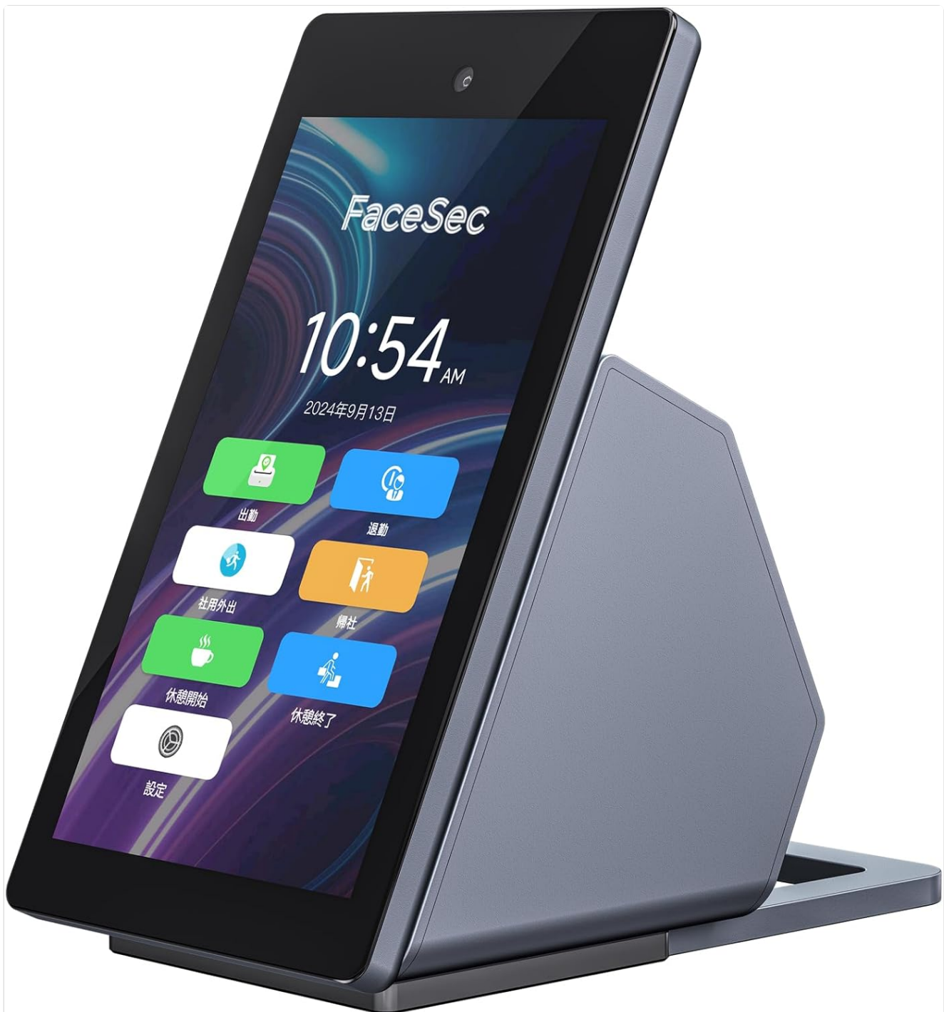
Figure 1.1: Front view of the FaceSec FAD-D55 device, showing the 5.5-inch touch display with the FaceSec logo and current time, along with various clock-in options.
