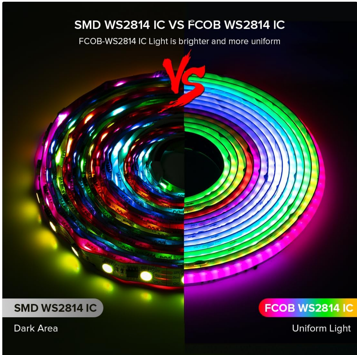
Image: Comparison showing the uniform light of FCOB WS2814 IC compared to the visible dots of SMD WS2814 IC.
