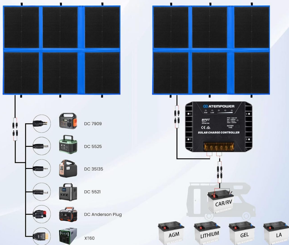
Image 4.2: Diagram illustrating the various connectors for compatibility with different power stations and battery types.
