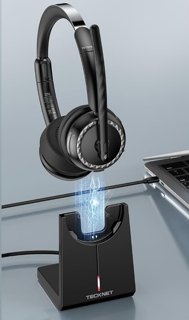
Image 2.2: Two charging methods: via dedicated base or direct Type-C cable.
