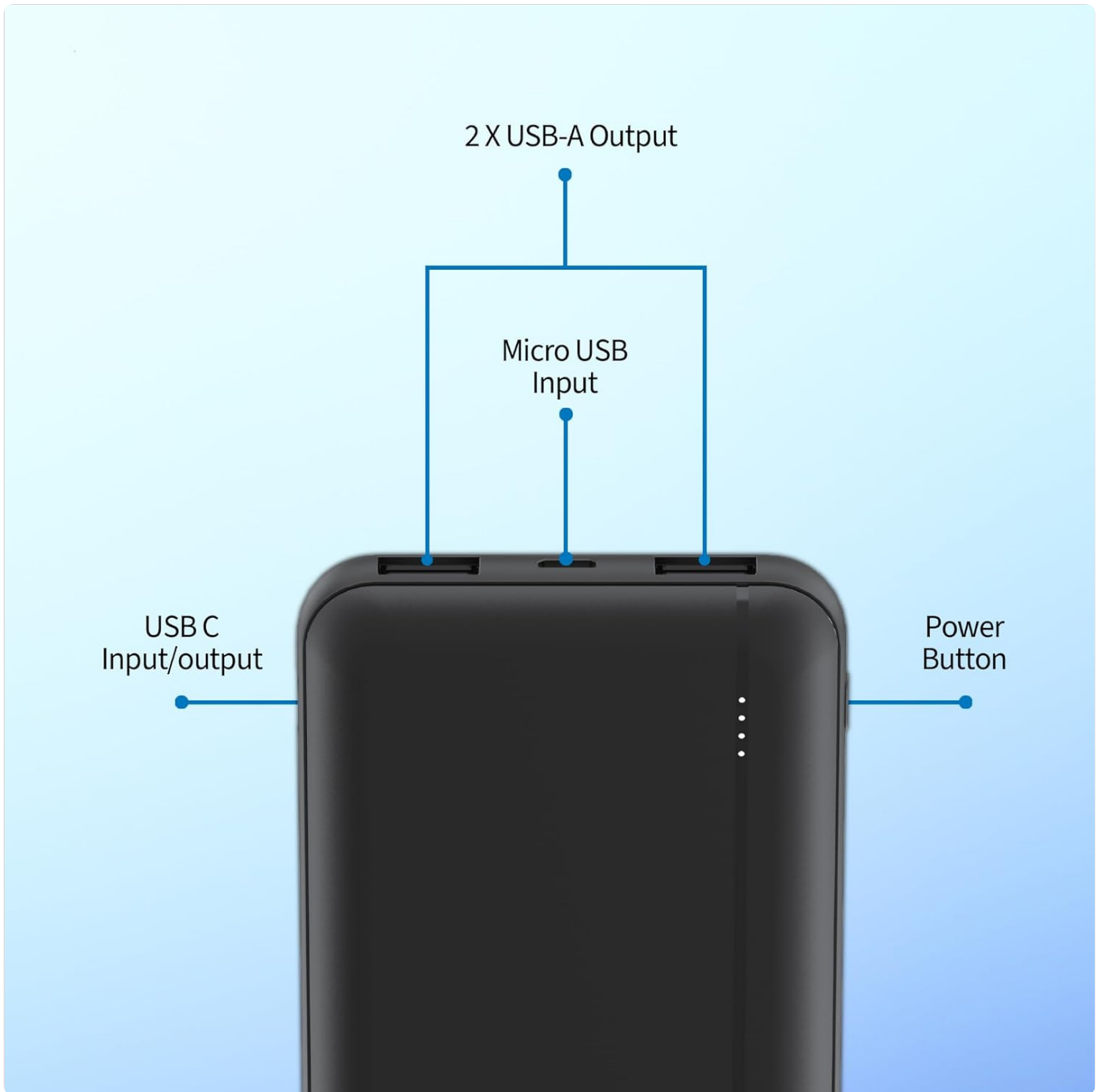
Image 2.1: Top view of the power bank highlighting its ports and button. From left to right: USB-C Input/Output port, Micro USB Input port, two USB-A Output ports, and the Power Button.
