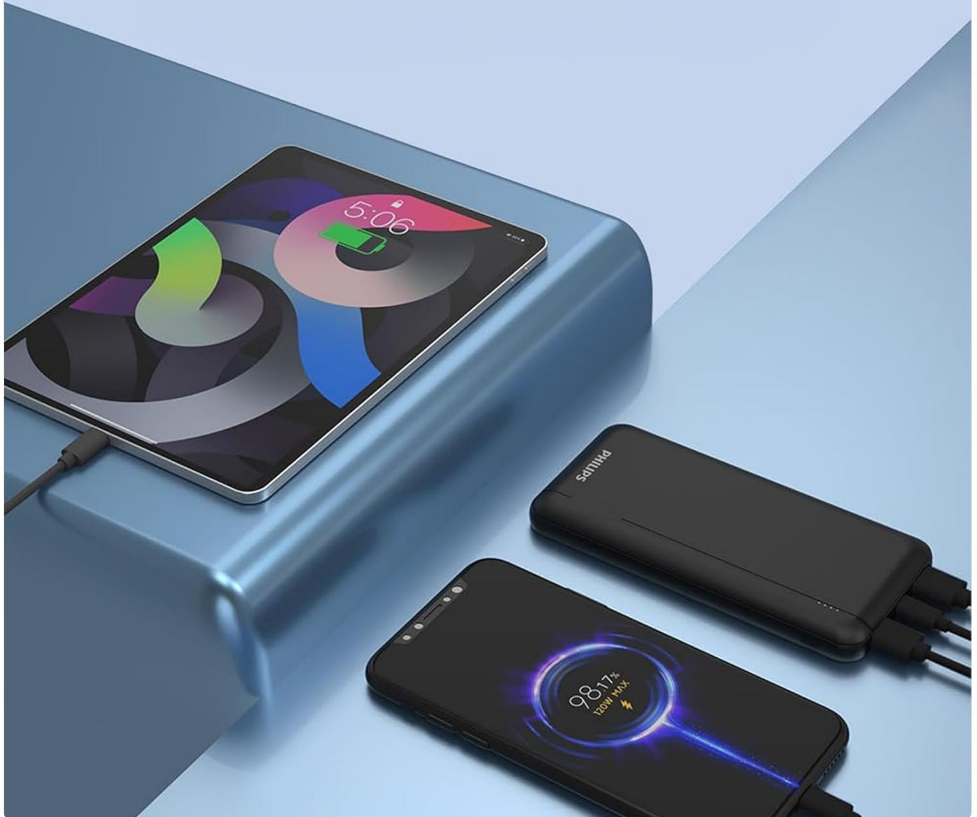
Image 4.1: The power bank simultaneously charging a tablet via its USB-C port and a smartphone via one of its USB-A ports, demonstrating its multi-device charging capability.
