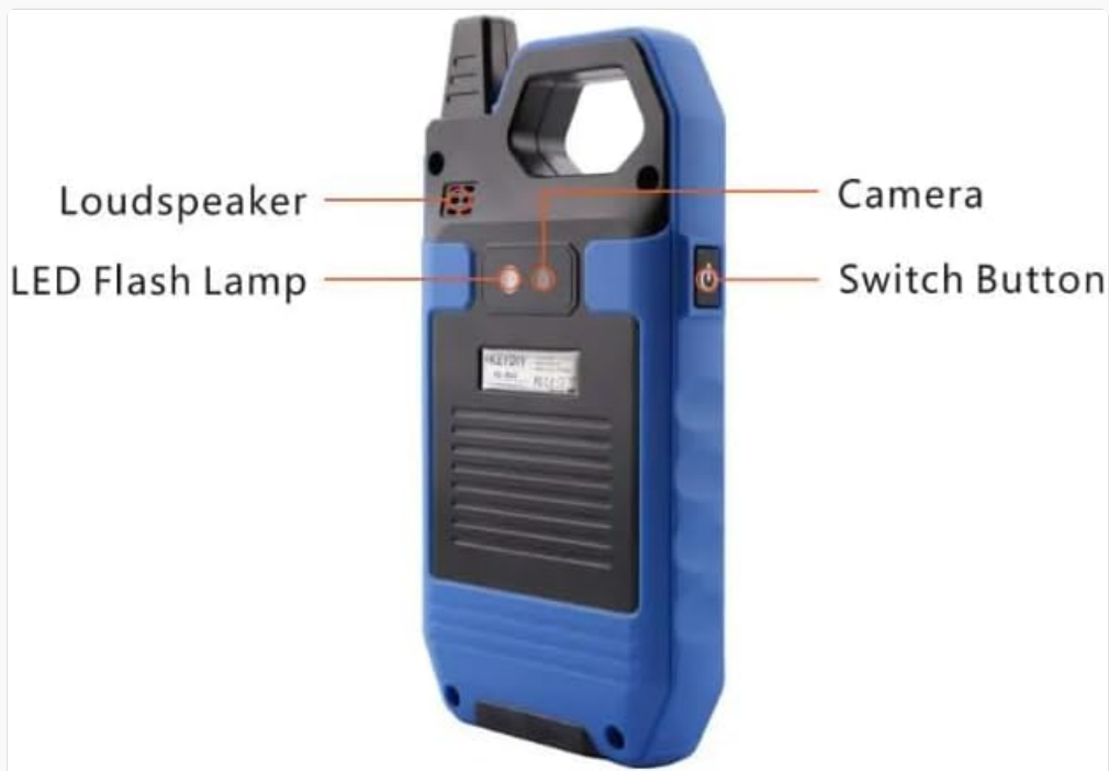
Image 2.1: Front and side view of the KDMAX device with labeled components.
