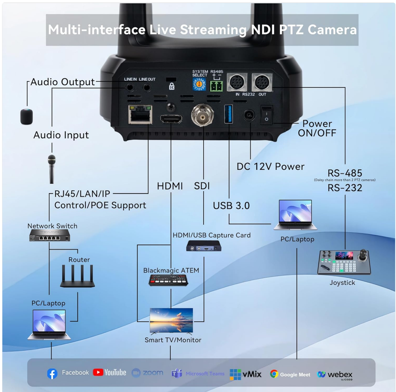
Figure 4: Detailed diagram of the camera's multi-interface connections and their typical uses.
