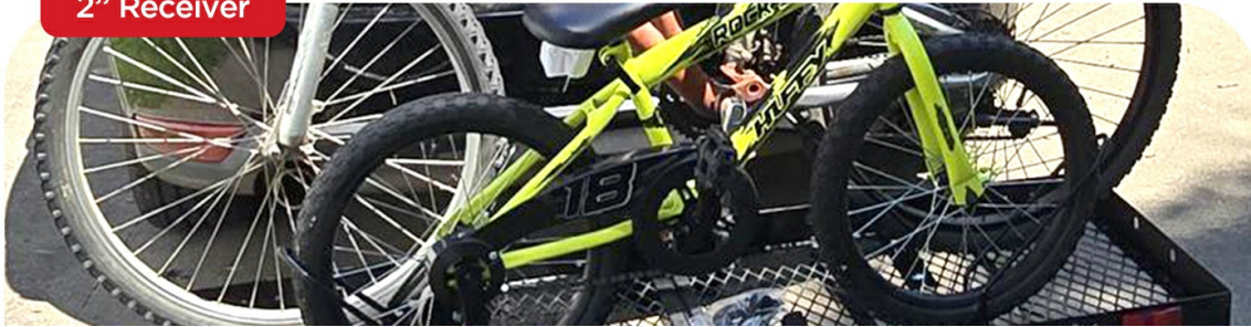
Image 4.1: The cargo carrier is designed to fit a standard 2-inch hitch receiver without drilling.
