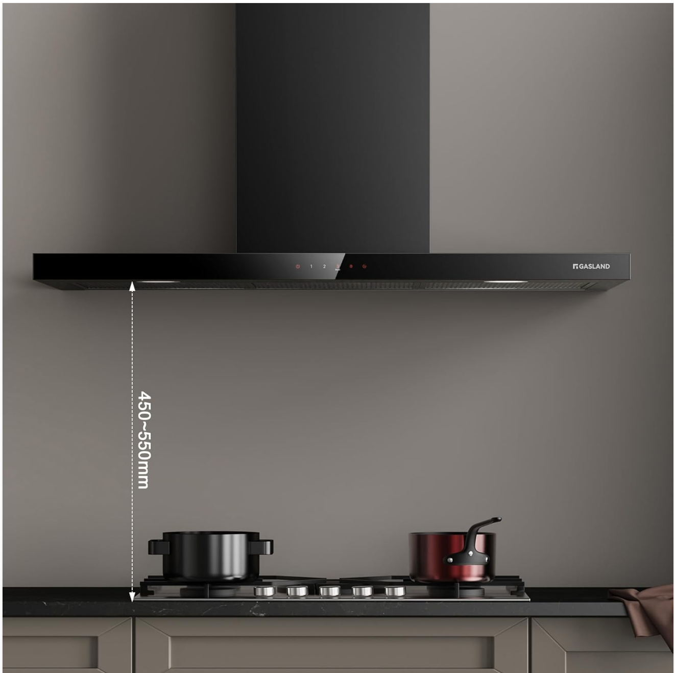
Image 2.2: Illustration showing the recommended installation height of 450-550mm between the cooking surface and the bottom edge of the range hood for optimal performance and safety.
