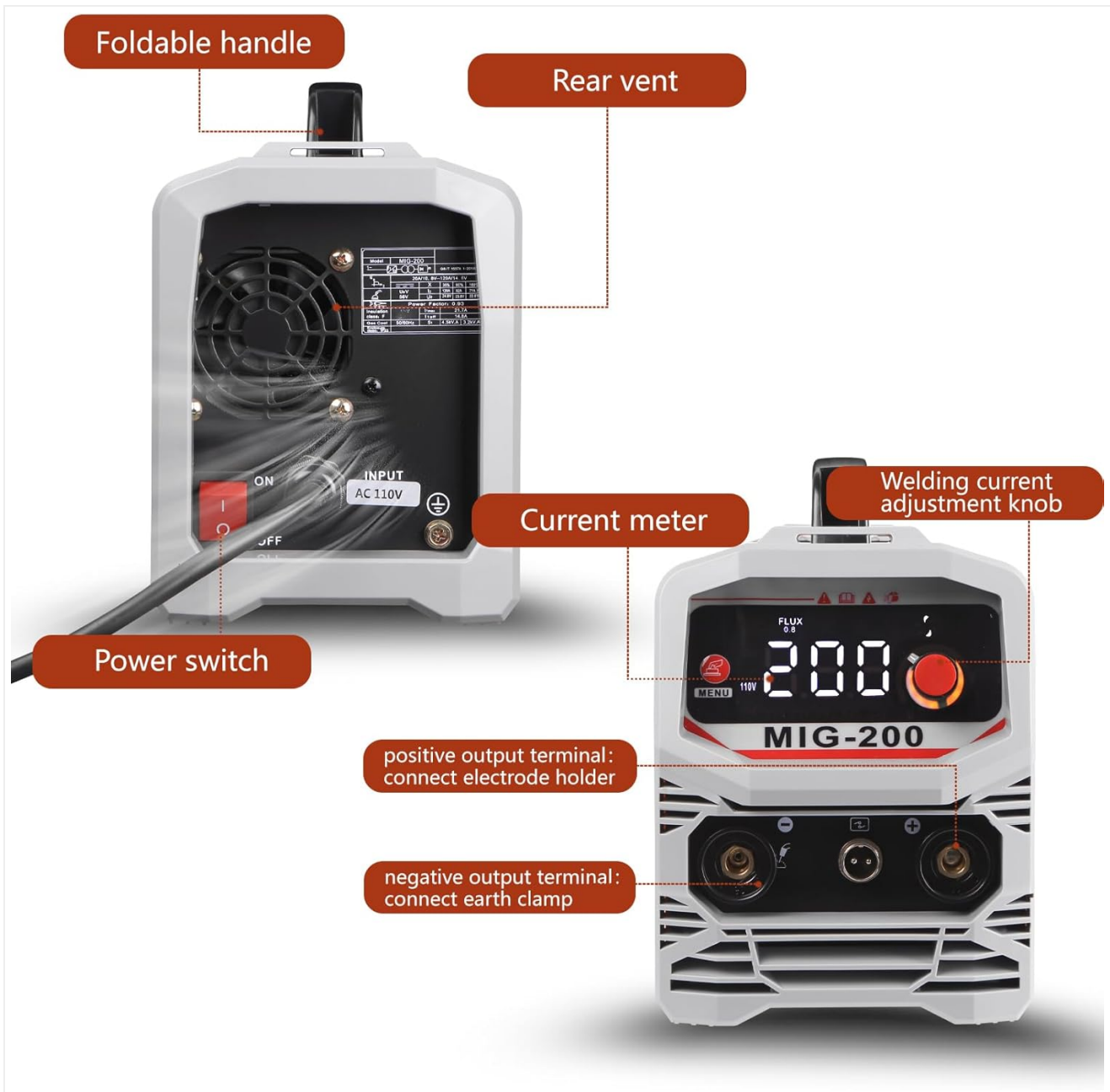
Figure 5: Detailed view of the MIG200's front panel, showing the welding current adjustment knob, current meter, positive output terminal for the electrode holder, and negative output terminal for the earth clamp. The rear panel shows the power switch and rear vent.
