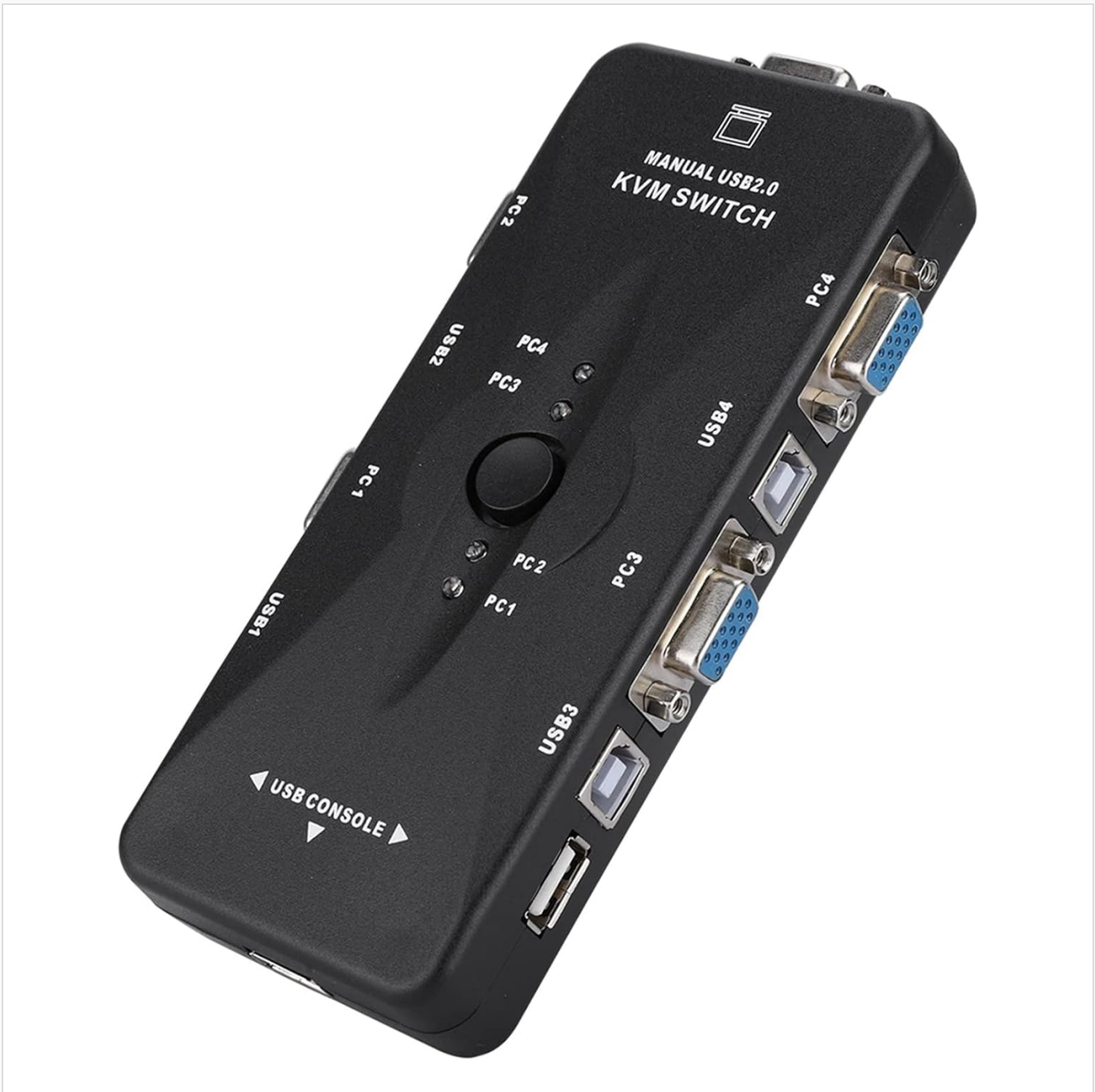
Figure 2: Top view of the KVM switch, highlighting the central selection button and LED indicators for active computer status.
