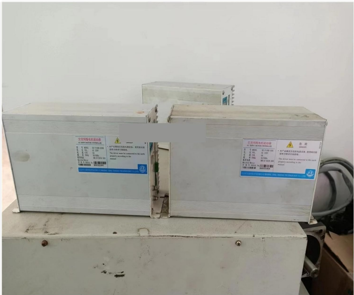
Figure 2: Side view of two Dahao AC Servo Motor Controller Drivers SD-P150. This image shows the side and top of two controller units, highlighting their compact form factor and the heat sink fins on the sides. Labels with technical specifications and warnings are visible on the top surface of the units.
